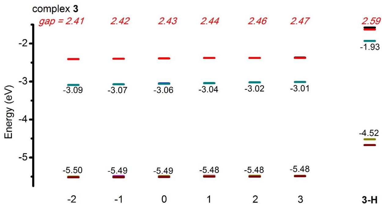
Figure S23 Plots of energy level of frontier orbitals in the lowest triplet states for 3 by changing the N–H bond length (-2, -1, 0, 1, 2, 3 denote the N–H bond length of 0.817, 0.917, 1.017, 1.117, 1.217, and 1.317 Å, respectively), in CH 2 Cl 2 solution by TDDFT method at the B3LYP level.
