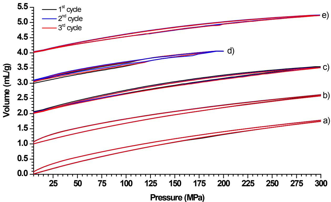
**Figure S4.** Pressure-volume diagrams of the a) “ZIF-7 crude–water”, b) “ZIF-7 activated–water”, c) “ZIF-90–water”, d) “Zn(dcim)<sub>2</sub>-SALE–water” and e) “ZIF-11–water” systems. For clarity the diagrams for each system are shifted by 1.0 mL/g along the y axis.
