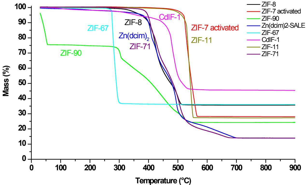
**Figure S2.** TG curves of ZIF-8 (black), activated ZIF-7 (red), ZIF-90 (green), Zn(dcim)<sub>2</sub>-SALE (blue), ZIF-67 (cyan), CdIF-1 (magenta), ZIF-11 (dark yellow) and ZIF-71 (purple) samples.
