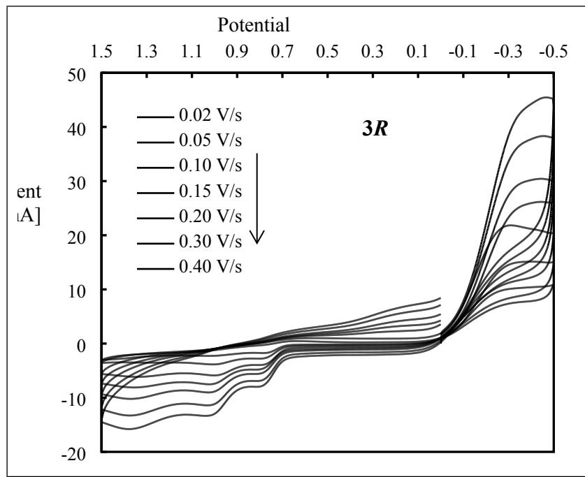
**Figure S2.** Cyclic voltammograms of **3R** (1.0 mmol/L); TBAP (0.1 mol/L) at varying scan rates in acetonitrile at 25 °C.
