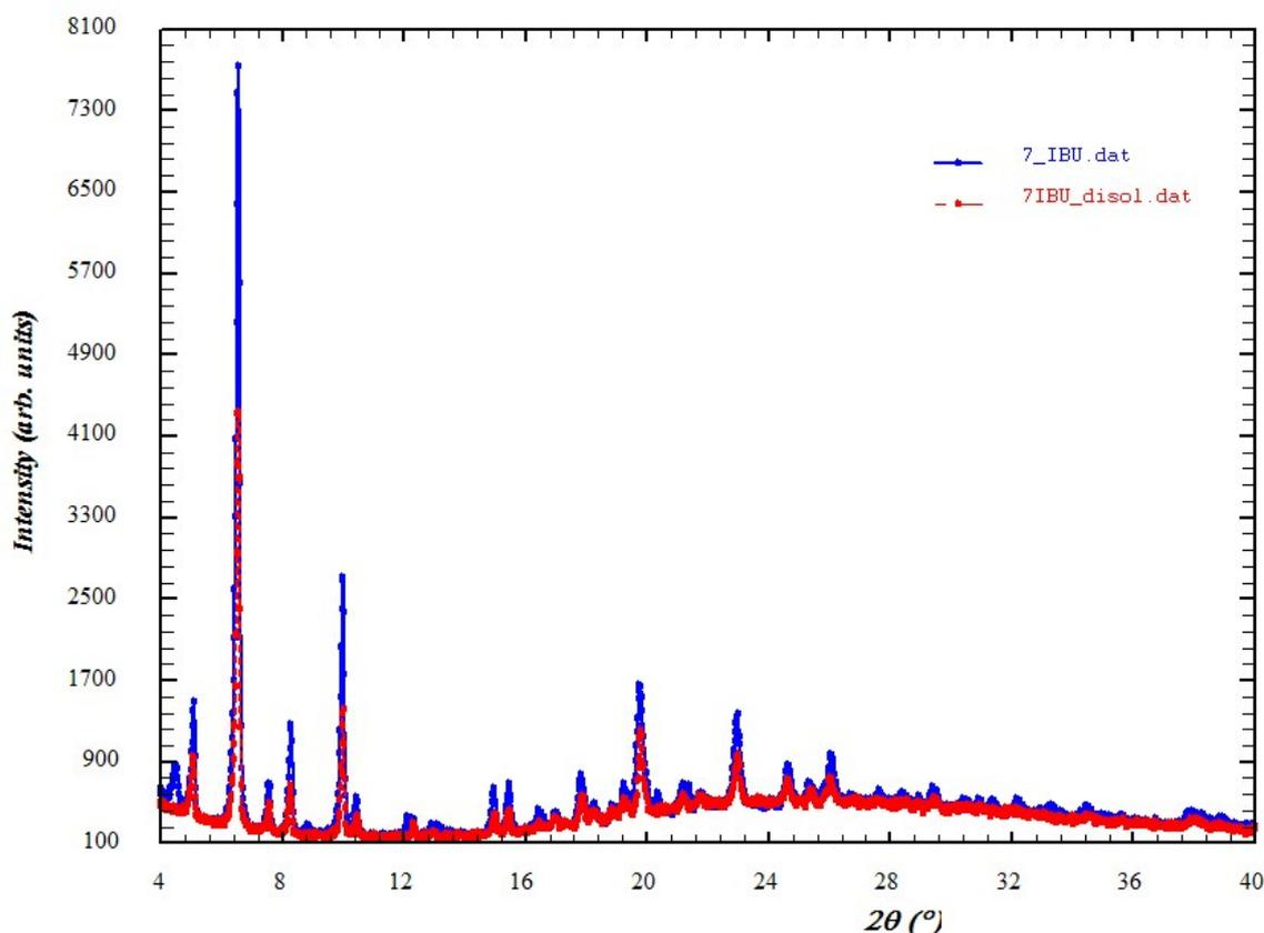
**Figure S3.** Powder X-ray diffractograms of **1** *before* (blue) and *after* (red) treatment with water.
