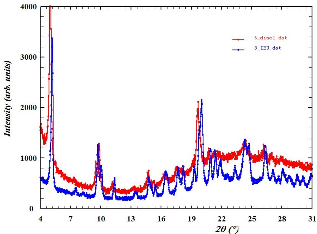
**Figure S4.** Powder X-ray diffractograms of **2** *before* (blue) and *after* (red) the treatment with water.
