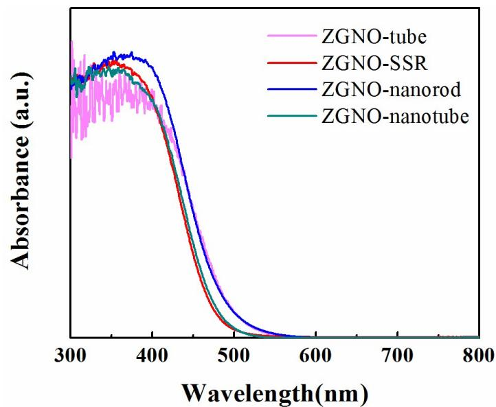
**Figure S4** UV-Vis absorption spectrum of ZGNO-SSR, ZGNO-tube, ZGNO-nanotube and ZGNO-nanorod.
