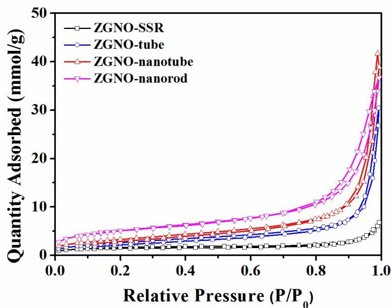
**Figure S3** The nitrogen adsorption-desorption isotherms of ZGNO-SSR, ZGNO-tube, ZGNO-nanotube and ZGNO-nanorod.
