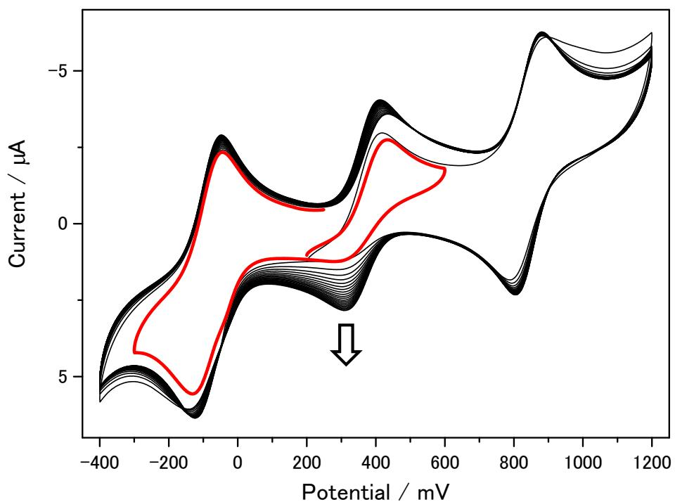
**Figure S5.** Cyclic voltammograms of  $K_7[\alpha_1\text{-P}_2\text{W}_{17}\text{O}_{61}\text{Ru}^{\text{III}}(\text{H}_2\text{O})]$  ( $\alpha_1\text{-RuH}_2\text{O}$ ) in Britton-Robinson buffer with 0.5 M  $\text{NaNO}_3$  solution (pH 6.0). (red line) potential window was between 600 mV and -300 mV. (black line) scans between 1200 mV and -400 mV were continually repeated 21 times. Potential scan was started from 200 mV to a positive direction.
