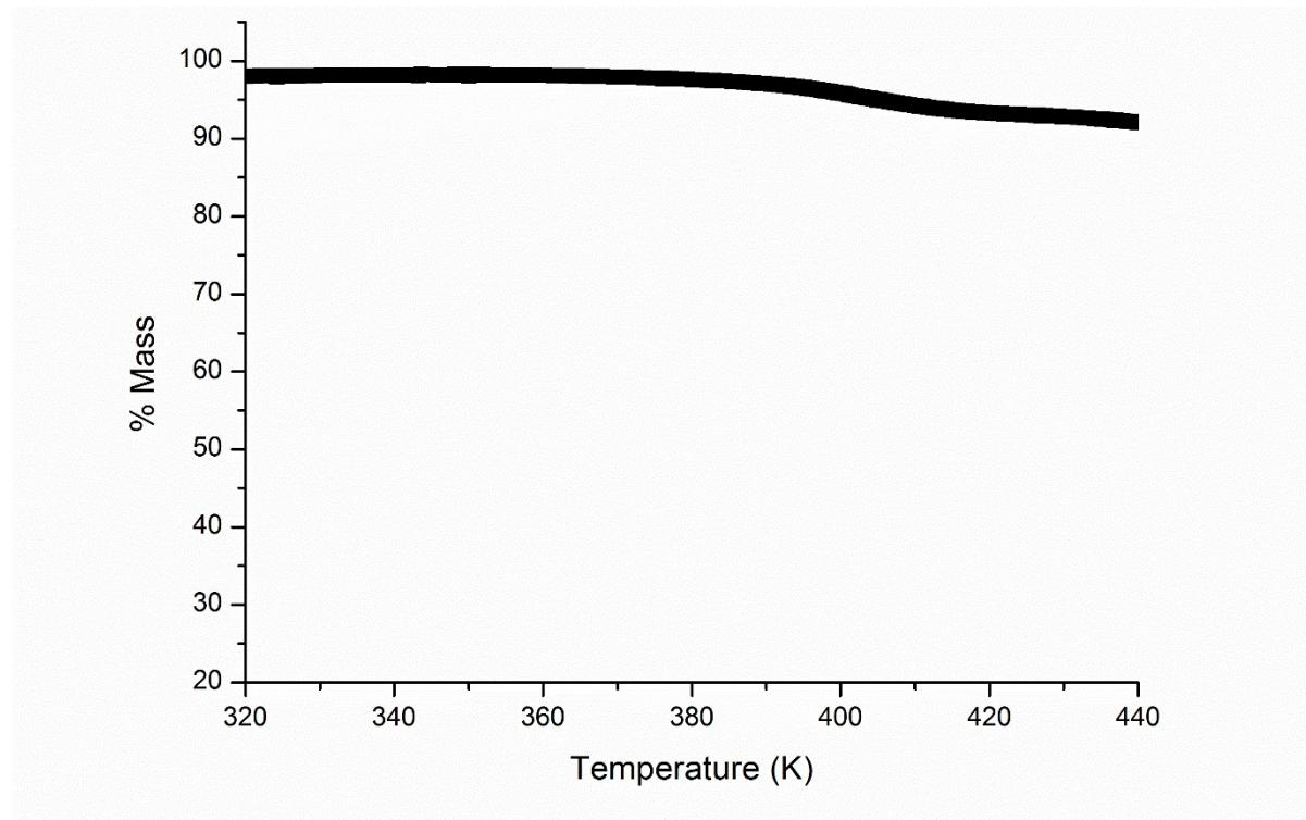
Fig. S2: Thermogravimetric Analysis of complex (**2**) showing water loss at 400 K.
