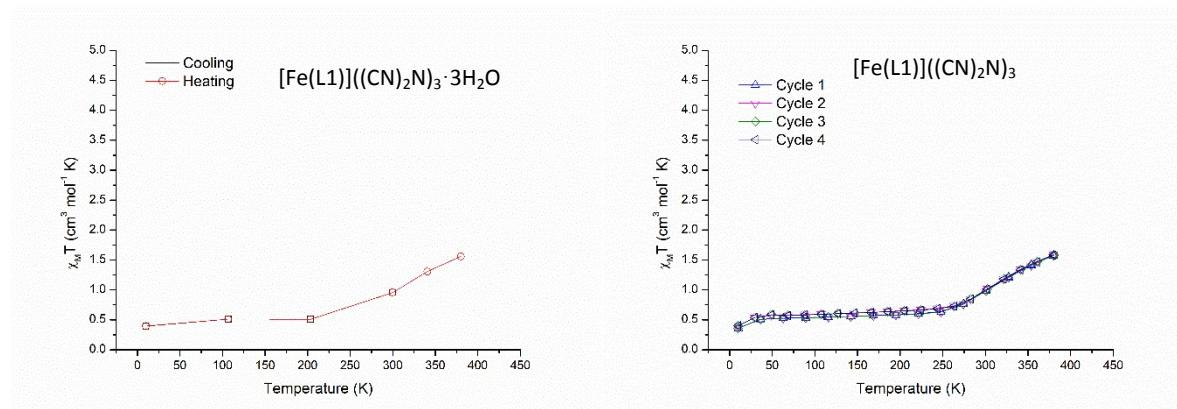
Fig. S1:  $\chi_M T$  v T plot for complex (**2**) and (**2'**), exhibiting change in the magnetic moment as a result of water loss.
