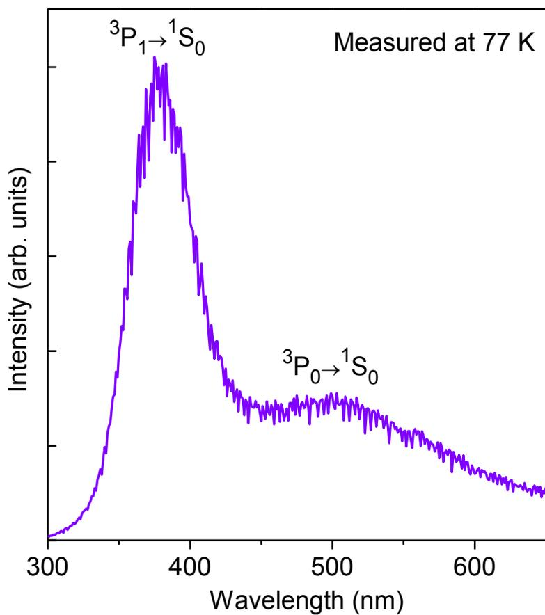
**Figure S2.** Photoluminescence emission spectrum of  $\text{Sr}_2\text{MgGe}_2\text{O}_7:\text{Pb}^{2+}$  persistent phosphor acquired under 280 nm light excitation at 77 K.
