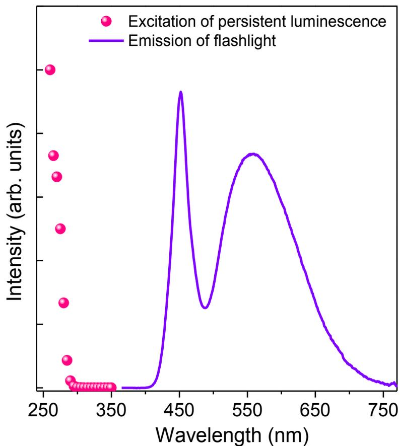
**Figure S3.** Emission spectrum of the white LED flashlight used in PSPL study. The flashlight is a YAG:Ce-based white LED with a output of  $\sim 1$  mW/cm<sup>2</sup>. The dots curve is the persistent luminescence excitation spectrum of the Sr<sub>2</sub>MgGe<sub>2</sub>O<sub>7</sub>:Pb<sup>2+</sup> phosphor, which is the same as the one in Fig. 2b. It is clear that the white LED cannot produce persistent luminescence in Sr<sub>2</sub>MgGe<sub>2</sub>O<sub>7</sub>:Pb<sup>2+</sup>.
