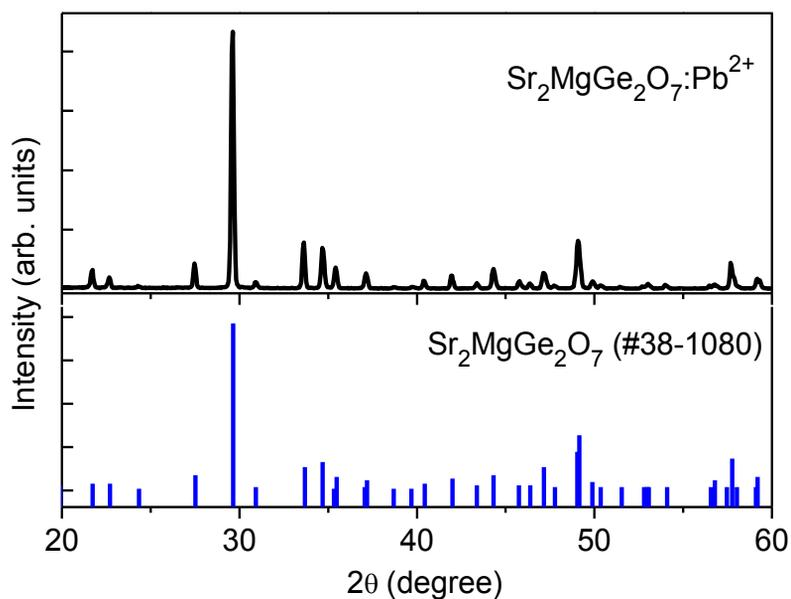
**Figure S1.** X-ray diffraction pattern of  $\text{Sr}_2\text{MgGe}_2\text{O}_7:0.5\%\text{Pb}$  phosphor. The pattern was acquired on a PANalytical X'Pert Pro X-ray diffractometer using  $\text{Cu K}\alpha_1$  radiation ( $\lambda = 1.5406 \text{ \AA}$ ). The bottom pattern is the indexation of melilite-structured  $\text{Sr}_2\text{MgGe}_2\text{O}_7$ .
