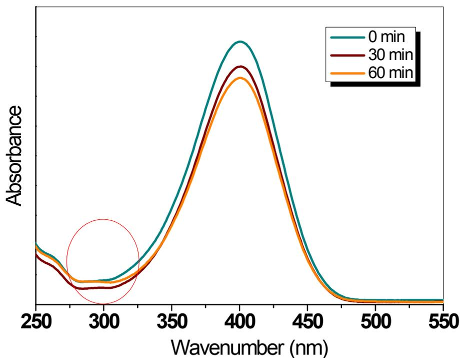
Figure 5. Successive UV-vis absorption spectra of the reduction of 4-NP by  $\text{NaBH}_4$  in the presence of  $\beta\text{-CD}$ . No peak around 300 nm was observed, suggesting that no 4-AP was formed.
