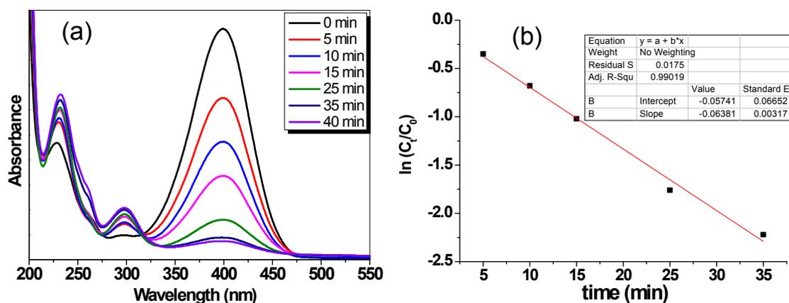
Figure 8. Successive UV-vis absorption spectra of the reduction of 4-NP by NaBH<sub>4</sub> in the presence of (a) Ru nanoparticles and (b) the logarithm of the absorbance at 400 nm vs. reaction time. (2 mg, 22 wt.% Ru by ICP, the other condition is the same as that of RuCu nanodendrites)
