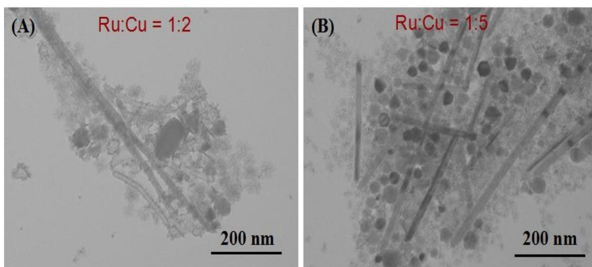
Figure 4. TEM images of RuCu products obtained with different molar ratio of  $\text{RuCl}_3 \cdot x\text{H}_2\text{O}$  and  $\text{CuCl}$  (A) 1:2 and (B) 1:5.
