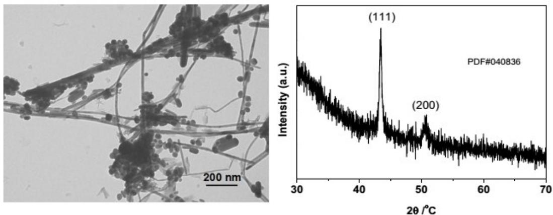
Figure 7. Metallic Cu obtained by CuCl and oleylamine. (Synthesis: 5 ml oleylamine and 10 mg CuCl at 473 K in an oil bath under stirring for 4 h)
