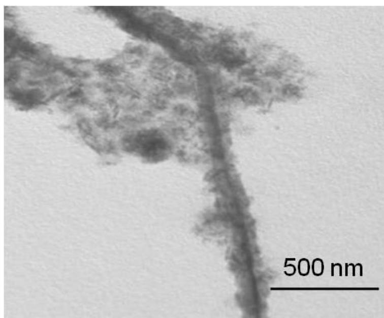
Figure 3. TEM images of RuCu products obtained with  $\text{RuCl}_3 \cdot x\text{H}_2\text{O}$  and  $\text{Cu}_2\text{O}$  at the ratio of 1:1.
