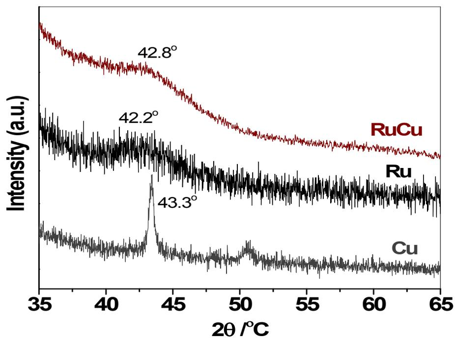
Figure 2. XRD patterns of RuCu nanodendrites, metallic Ru and metallic Cu.
