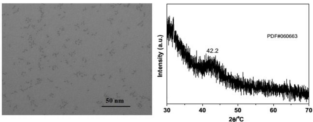
Figure 6. TEM images of Ru nanoparticles. (Synthesis: 10 ml ethylene glycol, 30 mg PVP(K-30) and 5 mg  $\text{RuCl}_3 \cdot x\text{H}_2\text{O}$  at 423 K in an oil bath for 4 h.)
