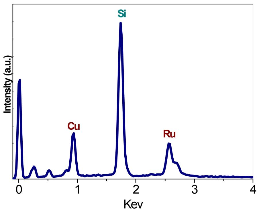
Figure 1. EDS result of RuCu nanodendrites.
