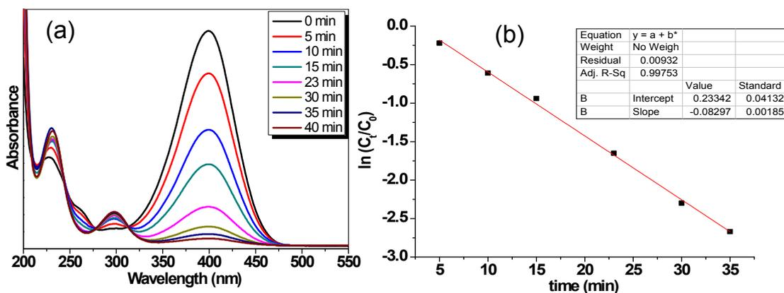
Figure 10. Successive UV-vis absorption spectra of the reduction of 4-NP by  $\text{NaBH}_4$  in the presence of (a) physical mixtures Ru nanoparticles as well as metallic Cu and (b) the logarithm of the absorbance at 400 nm vs. reaction time. (2 mg Cu catalyst and 2 mg Ru catalyst, the other condition is the same as that of RuCu nanodendrites)
