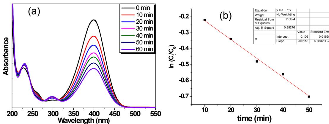
Figure 9. Successive UV-vis absorption spectra of the reduction of 4-NP by  $\text{NaBH}_4$  in the presence of (a) metallic Cu and (b) the logarithm of the absorbance at 400 nm vs. reaction time. (2 mg, 23 wt.% Cu by ICP, the other condition is the same as that of RuCu nanodendrites)
