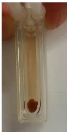
**Fig. S26:** Picture of the alginate spheres on the bottom of a temperature controllable UV/VIS cell with myoglobin solution.
