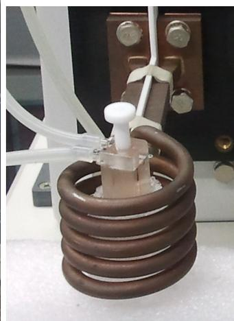
**Fig. S40** Setup of the CO release measurements in alternating current (AC) field with a Hüttinger HF generator AXIO T5 and the thermostated quartz cell placed inside the water-cooled copper induction coil.
