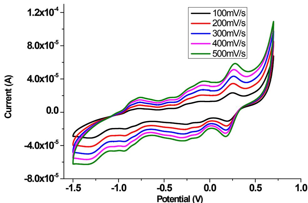
**Fig S5** Cyclic voltammograms of  $2.5 \times 10^{-5}$  M solution of **1** in  $\text{CH}_3\text{CN}$  with different scan rates. The working electrode was glassy carbon, the counter electrode was Pt wire, and the reference electrode was Ag/AgCl
