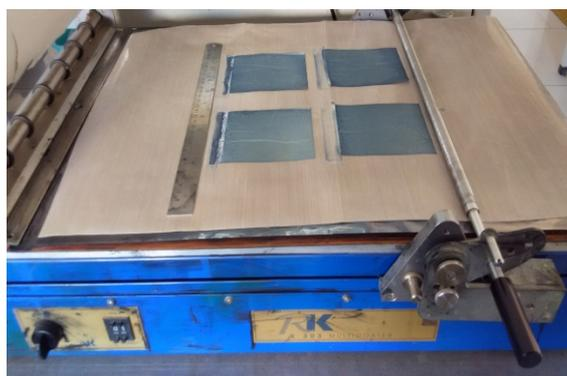
Figure S13 . Preparation of four PEDOT-p-1 of 100  $\text{cm}^2$  simultaneously using roll coat methode.
