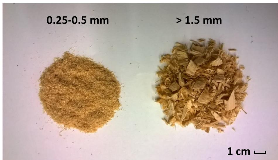
**Fig. S1** Comparison between fine-milled birch sawdust (0.25-0.50 mm), the standard reaction substrate, and the larger fraction (> 1.5 mm) of birch sawdust, which was tested with regard to its potentially reduced milling cost.
