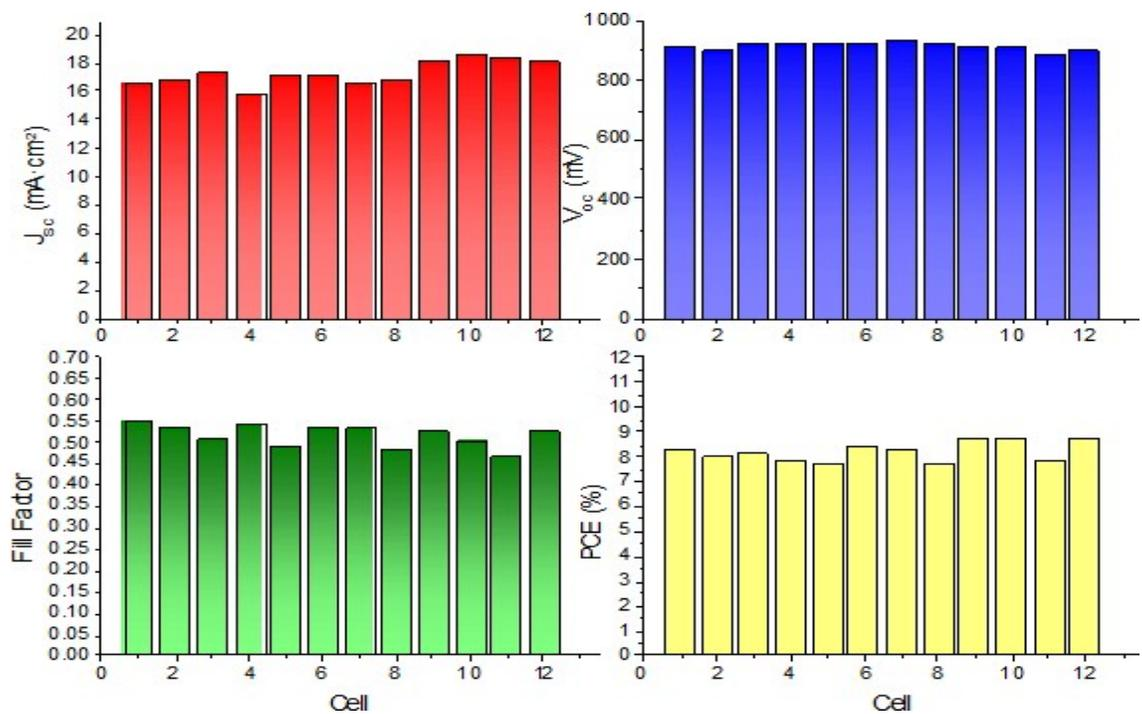
Figure S11: Statistical data of the devices, where doped TIPS-pentacene, was solution processed in toluene and used as an HTM layer.
