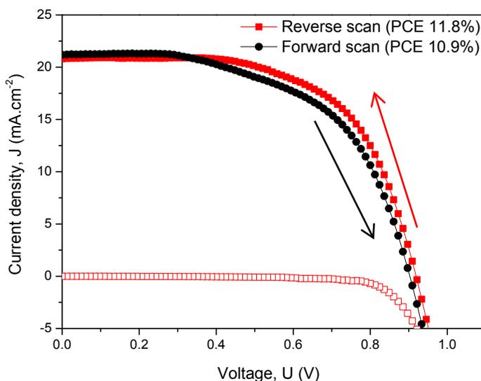
Figure S6: Current-voltage characteristics of champion device prepared with pristine TIPS-pentacene as HTM measured in forward (from short circuit current to open circuit voltage) and reverse (from open circuit voltage to short circuit current) bias scan.
