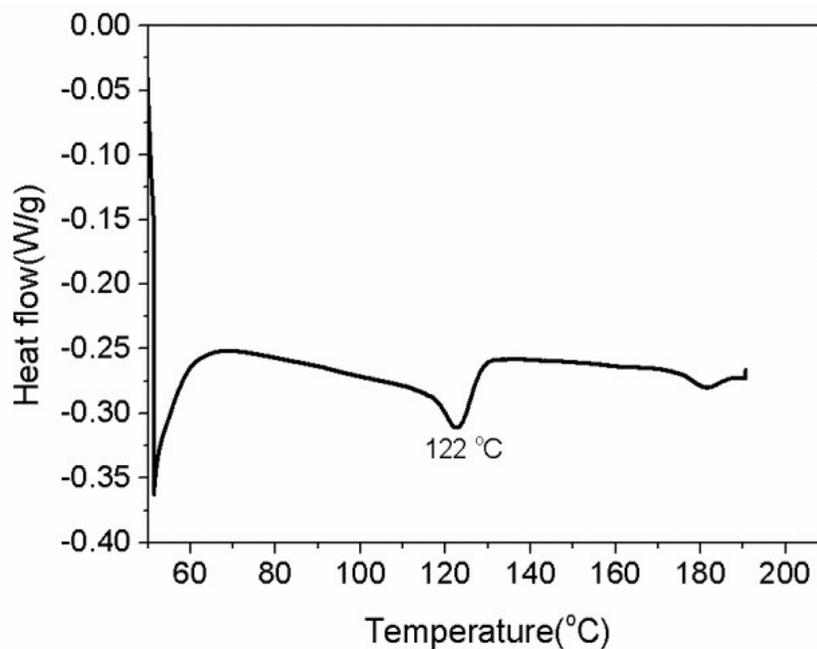
Figure S2 : Differential Scanning Calorimetry (DSC) measurement for TIPS-pentacene at a scan rate 5°K/min in nitrogen atmosphere.
