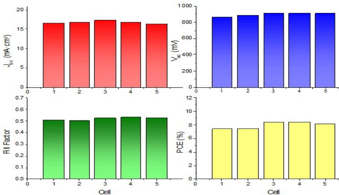
Figure S13 : Statistical data of the devices, where doped TIPS-pentacene, was solution processed in chlorobenzene and used as an HTM layer.
