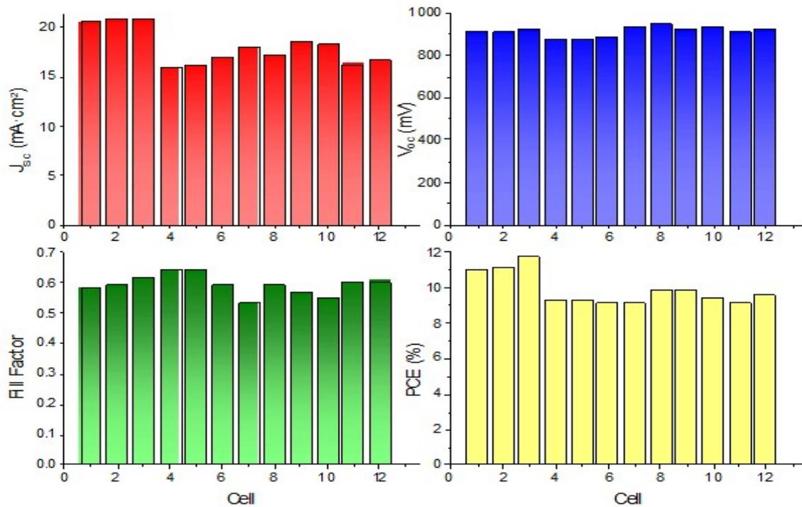
Figure S10: Statistical data of the devices, where TIPS-pentacene was solution processed in toluene and used as an HTM layer.
