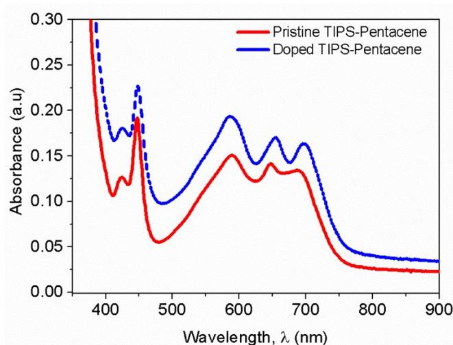
Figure S1: UV-Vis absorbance spectra of TIPS-pentacene film on quartz substrate.
