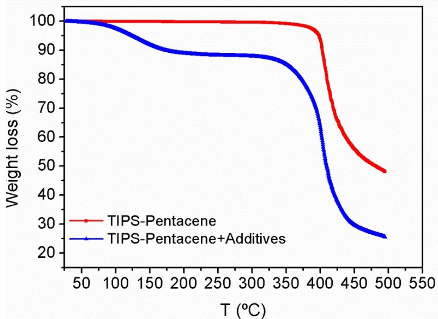
Figure S3 : Thermogravimetric analysis (TGA) of pristine TIPS-pentacene and with LiTFSI and t-BP as additive with scan rate of 10°K·min<sup>-1</sup>. Pristine TIPS-pentacene is more stable up to temperatures of around 380°C, while the one with additive shows stability up to 330°C.
