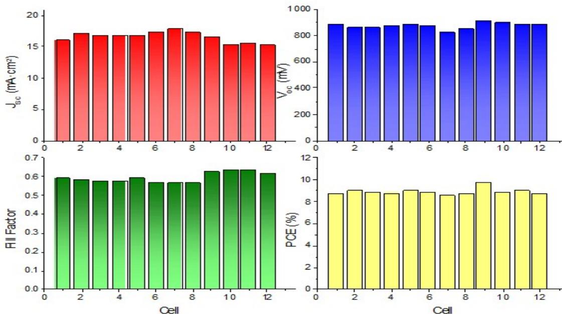
Figure S12: Statistical data of the devices, where TIPS-pentacene was solution processed in chlorobenzene and used as an HTM layer.
