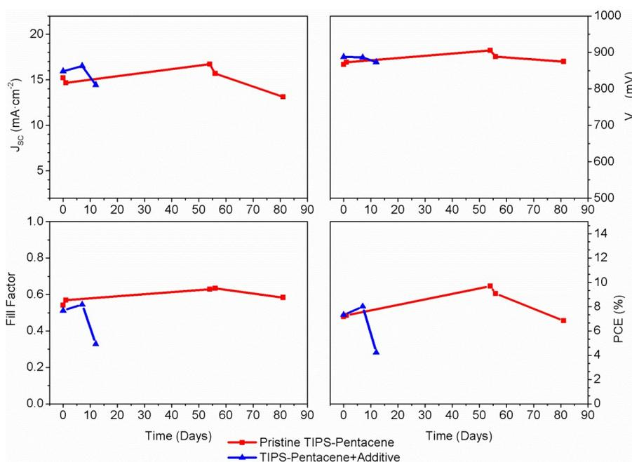
Figure S9 : Evolution of device parameters with time. Devices were kept in drybox and the efficiencies were measured by taking them out on then returned it back in the drybox.
