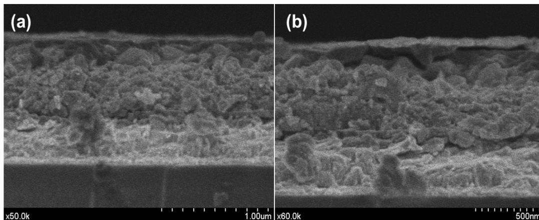
Figure S4 : Cross-sectional SEM image of the  $\text{CH}_3\text{NH}_3\text{PbI}_3$  perovskite based devices with doped TIPS-pentacene HTM, (a) at 1- $\mu\text{m}$  scale with low magnification and (b) at 500 nm scale with high magnification. Not so well defined or sharp interface between TIPS-pentacene and perovskite layer can be observed.
