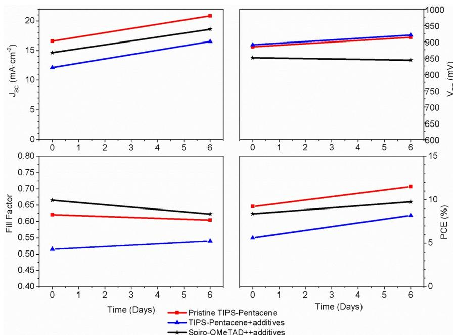
Figure S8 : Aging effect in pristine TIPS-Pentacene, doped TIPS-Pentacene and doped spiro-OMeTAD based devices.
