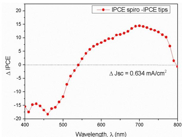
Figure S7. Difference of IPCE spectra ( $\Delta\text{IPCE} = \text{IPCE}_{\text{spiro}} - \text{IPCE}_{\text{(pristine TIPS-pentacene)}}$ ). The difference in IPCE results in a difference of  $J_{\text{sc}}$  of about  $0.63 \text{ mA/cm}^2$ .
