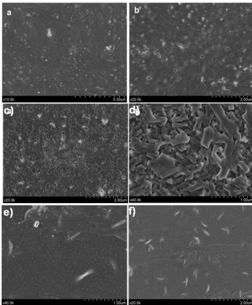
Figure S5: a-b) Surface morphology (top view) of pristine TIPS-pentacene based devices, c-d) morphology of doped TIPS-pentacene and e-f) surface morphology (top view) of doped spiro-OMeTAD based devices at low and high magnification.
