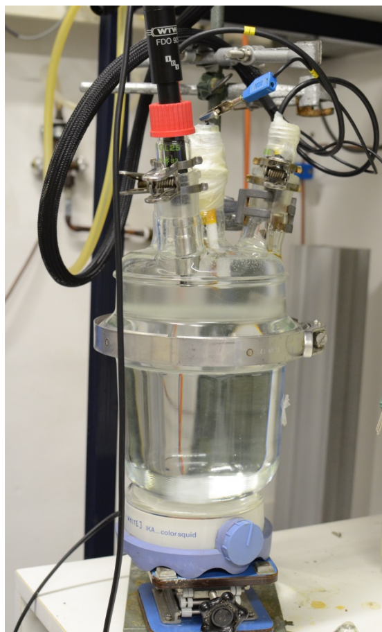
Figure S3: The set-up used for determining the Faradaic efficiency. Volume of the vessel: 2.3l. Dissolved oxygen was determined with an optical sensor using the fluorescence quenching method (Multi 3420 IDS from WTW, Weilheim, Germany). The Faradaic efficiency of sample Elox300 was determined at current densities of 10 mA/cm 2 and at 1 mA/cm 2 at 260, respectively 215 mV overpotential in 0.1 M KOH after 4000 respectively after 60000 s runtime. The results can be taken from Table S2, respectively from Figure 1c (measurement at 10 mA/cm 2 ).
