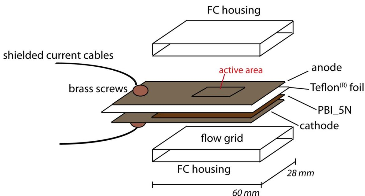
**Fig. S3** Exploded view of the MEA inside the FC housing. The MEA is constituted by four foils in this order from up to bottom: anode, Teflon<sup>®</sup> foil, PBI\_5N membrane and cathode. The two electrodes are longer than the Teflon<sup>®</sup> cylinder in order to allow a direct connection with the
