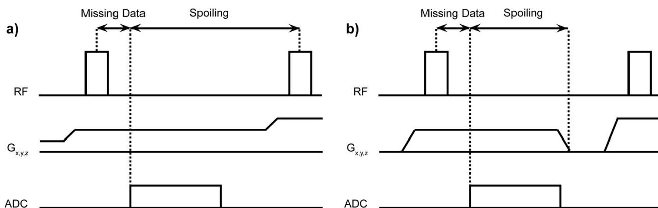
**Fig. S4** Schemes of the ZTE acquisition protocol. If the minimum  $T_R$  is used the gradient are always on (case a), otherwise they are switched on and off like in spin echo sequence (case b). [Scheme courtesy from Bruker Biospin GmbH].
