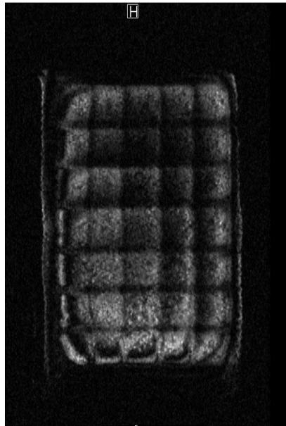
**Fig. S8** Preliminary test with a phantom of the surface coil: MRI image obtained for a rectangle of wet filter paper (2D spin echo sequence, coronal slice (3 x 4 cm, thickness 1 mm,  $T_R = 0.6s$ ,  $T_E = 14ms$ , matrix 256 x 256).
