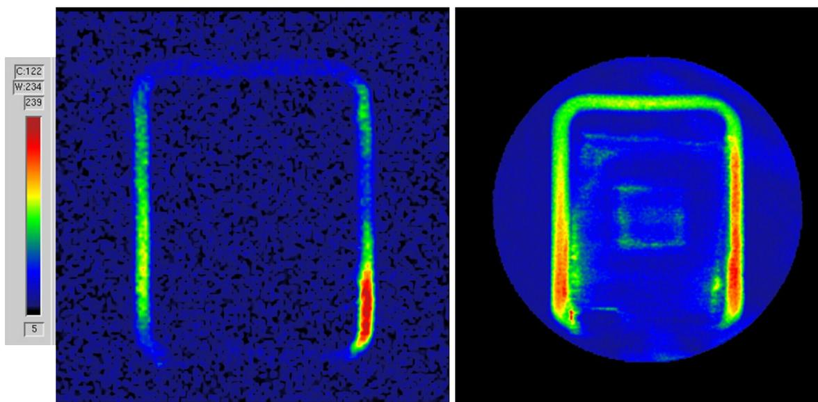
**Fig. S9** Preliminary tests with a MEA: left) a 2D spin echo image (coronal 4x4cm, thickness 5 mm,  $T_E=3.1\text{ms}$ ,  $T_R=1\text{s}$ ,  $N_A=4$ , 128x128 matrix, 0.312 mm/pixel); right) ZTE image (coronal 4x4x4cm,  $T_R=4\text{ms}$   $N_A=4$ , 192x192x192 0.208 mm/pixel).
