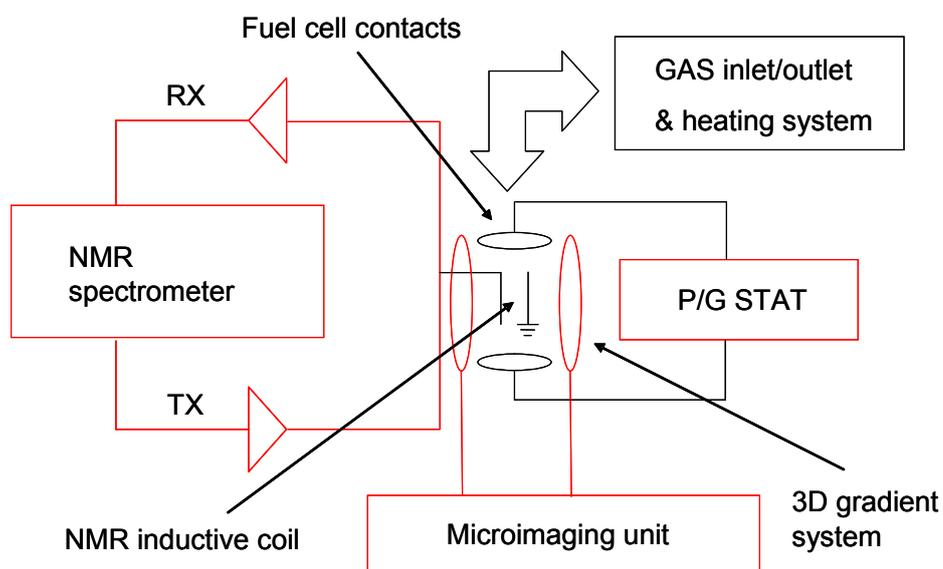
**Fig. S1** Block scheme of the ELMINMR instrument. Red: commercially-available parts, black parts: homemade or partially modified parts.
