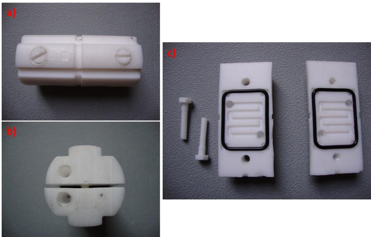
**Fig. S2** Teflon housing for MEA: a) lateral view; b) sectional view, where the two big holes are gas inlets, whereas the small hole is the thermocouple inlet; c) exploded view of the housing with the gas-flow channels and the o-rings.
