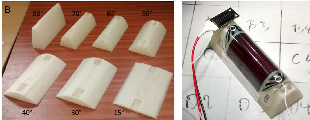
Fig. SI-2(a) (left) Substrates used for experiments and (right) image of a module mounted onto the corrugated substrate
