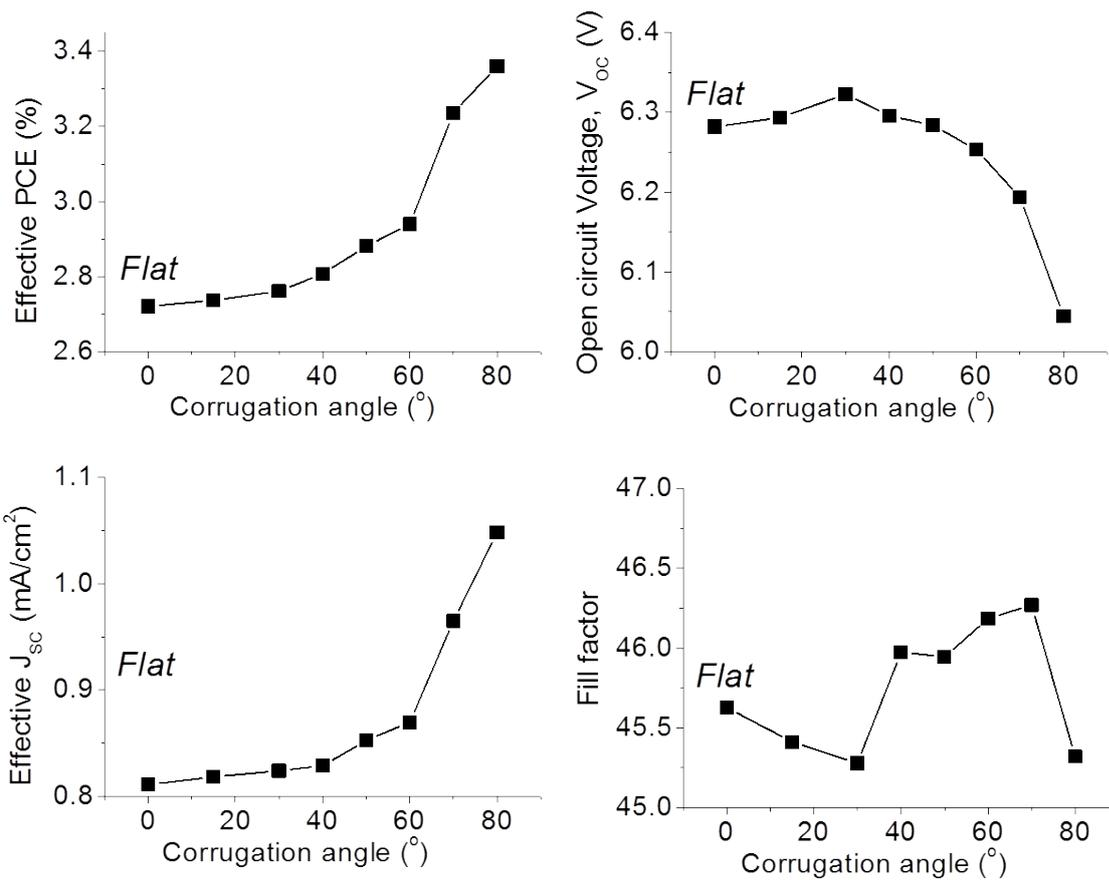
Figure SI-2(b) Effect of corrugation angle on (top left) Effective PCE (top right)  $V_{OC}$  (bottom left) Effective  $J_{SC}$  and (bottom right) FF.
