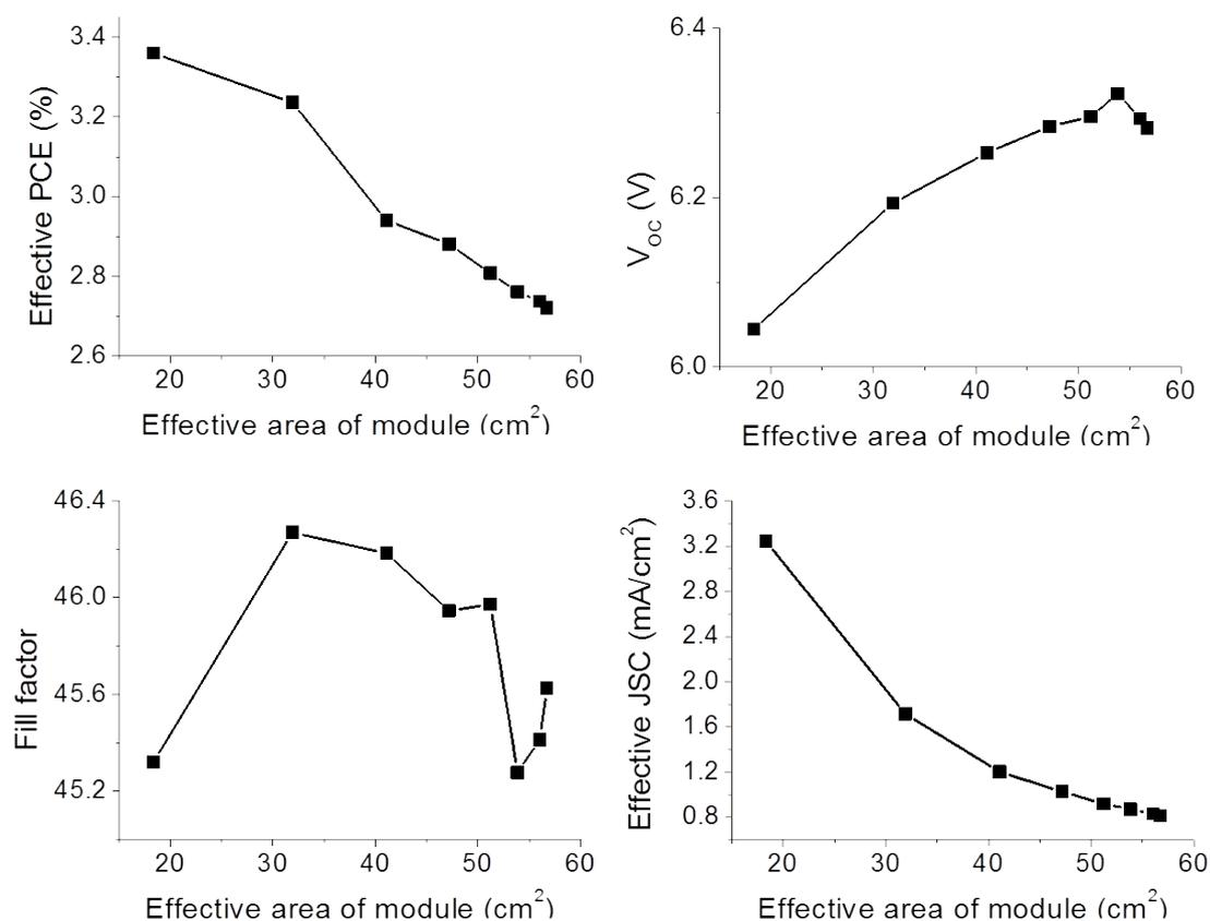
Figure SI-2(b) Effect of module footprint ('effective area') on (top left) Effective PCE (top right) V<sub>OC</sub> (bottom left) Effective JSC and (bottom right) FF.
