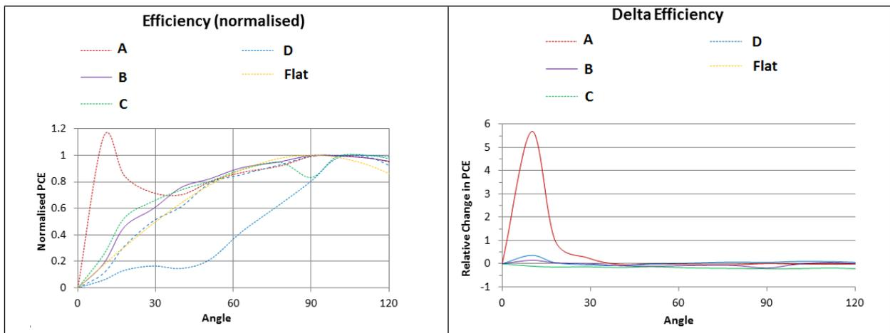
**SI-5 Raytracing simulation of enhancement in performance**
