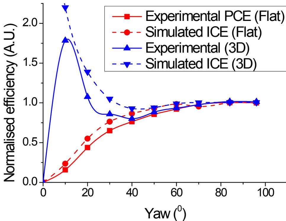
Figure SI-5b Experimental PCE data of the flat and Module A (pitch= 0°) as a function of yaw. Overlaid is the simulated in-coupling efficiency (ICE) of the flat module and Module A.
