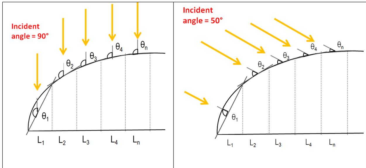
Figure SI-5a Schematic of the device used for simulation showing how the angles and lengths are calculated at incident angle ('yaw') =  $50^\circ$  (i.e. under normal incidence) and (right) at incident angle =  $50^\circ$ . The program simulates the in-coupling of light into a flat or corrugated module, which is the major loss mechanism to affect the photocurrent and efficiency.
