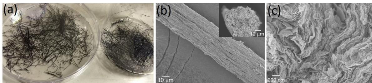
**Figure S2.** (a) Photograph of rGO fibers synthesized using space confinement fillers containing cylindrical channels of 0.5 mm in diameter. (b) SEM images of the dried rGO fiber with its fracture end area shown in the inserted image. (c) An enlarged view of fracture end area of the rGO fiber.
