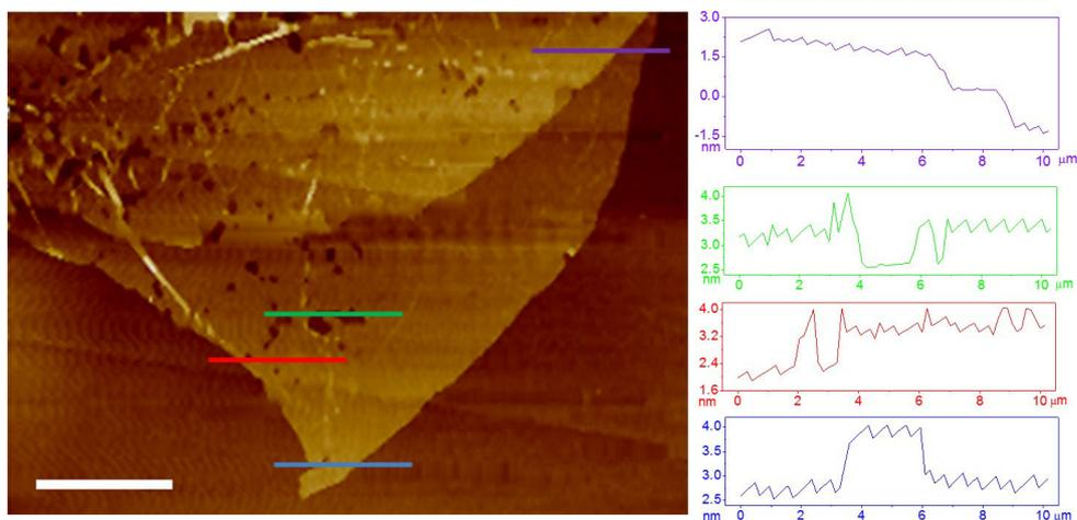
**Figure S1.** A typical AFM image of GO sheets used in this work. Height profiles on the right side were obtained along the marked straight lines in different colors on the AFM image. Scale bar in the AFM image is 10  $\mu\text{m}$ .
