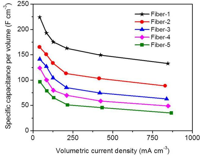
**Figure S10.** Specific volumetric capacitances of hybrid carbon fibers calculated from their GC curves as a function of the volumetric charge/discharge current density.
