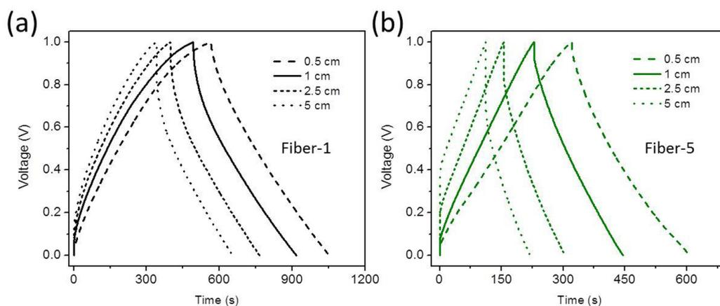
**Figure S12.** GC curves the fiber-based micro-SCs assembled using the rGO/MWCNT hybrid (a) fiber-1 and (b) fiber-5 in different lengths of 0.5, 1, 2.5, and 5 cm. All measurements were carried out under the same volumetric current density of about  $85 \text{ mA cm}^{-3}$ . The actual currents used were adjusted according to the total volume of each micro-SC (Table S1).
