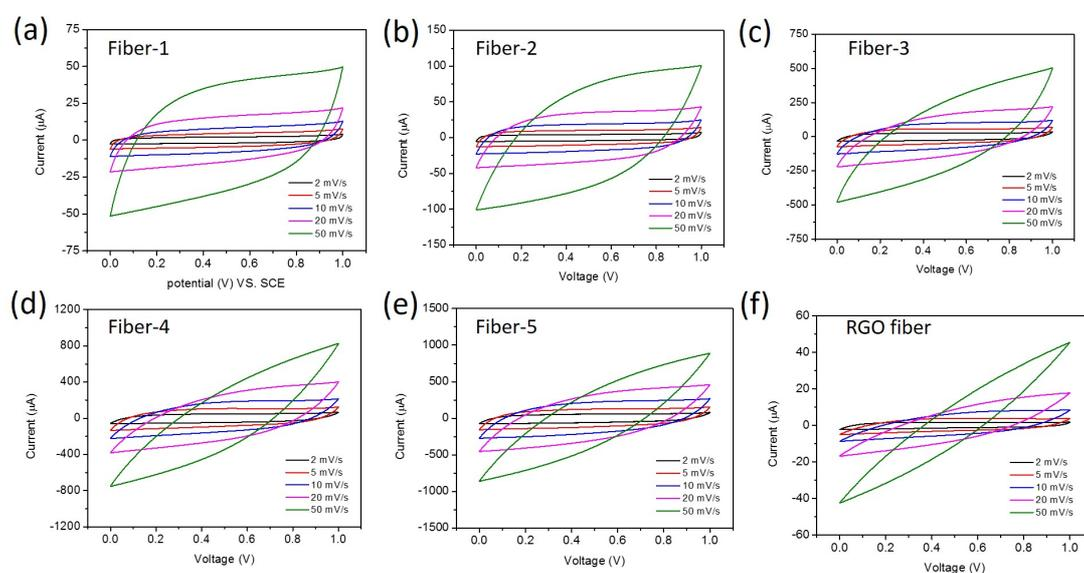
**Figure S7.** CV curves of fiber-based solid-state micro-SCs assembled using rGO fiber and rGO/MWCNT hybrid fibers in different diameters. The CV curves were measured at the scan rates from 2 to 50 mV/s.
