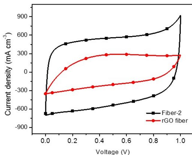
**Figure S8.** CV curve of fiber-based solid-state micro-SCs assembled using rGO fiber and fiber-2 at  $5 \text{ mV s}^{-1}$ .
