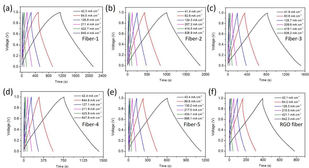
**Figure S9.** GC curves of the fiber-based solid-state micro-SCs assembled using the rGO fiber and rGO/MWCNT hybrid fibers in different diameters. The GV curves were measured at different charge/discharge current densities specified in the individual figures.
