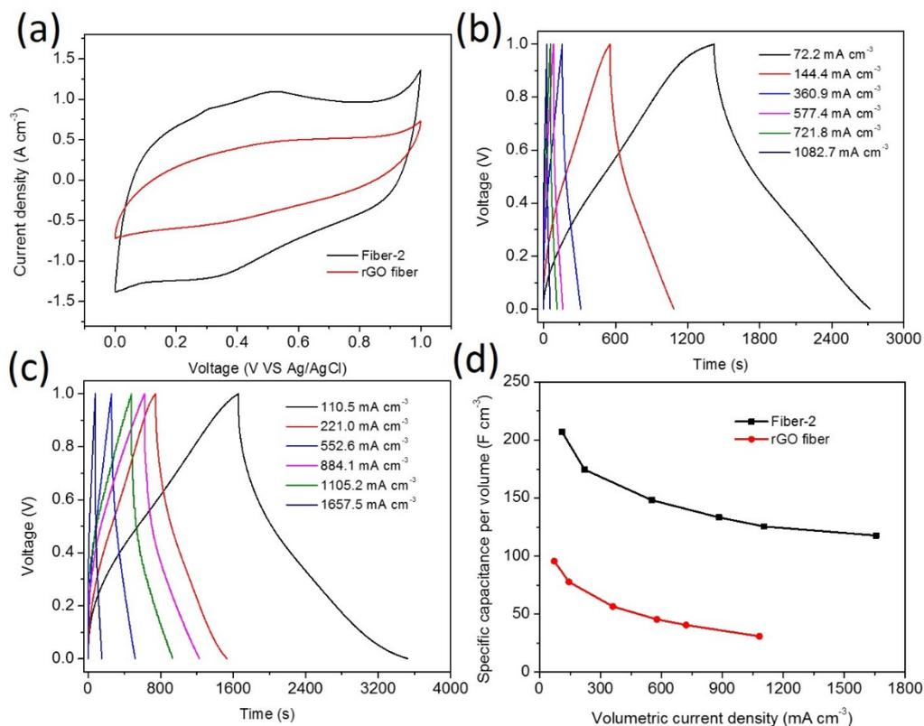
**Figure S6.** Electrochemical performances of fiber-2 and the rGO fiber measured using a three-electrode cell in 1 M H<sub>2</sub>SO<sub>4</sub> electrolyte. (a) CV curve measured at the scan rate of 5 mV s<sup>-1</sup>. GC curves of the (b) rGO fiber and (c) fiber-2 at different current densities. (d) Specific volumetric capacitance of fiber-2 and the rGO fiber as a function of charge/discharge current density calculated from their GC curves.
