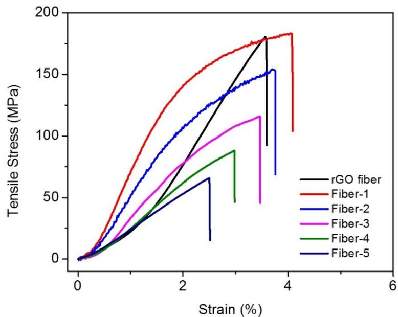
**Figure S3.** Stress-strain profiles of rGO fiber and rGO/MWCNT hybrid fibers in five different diameters.
