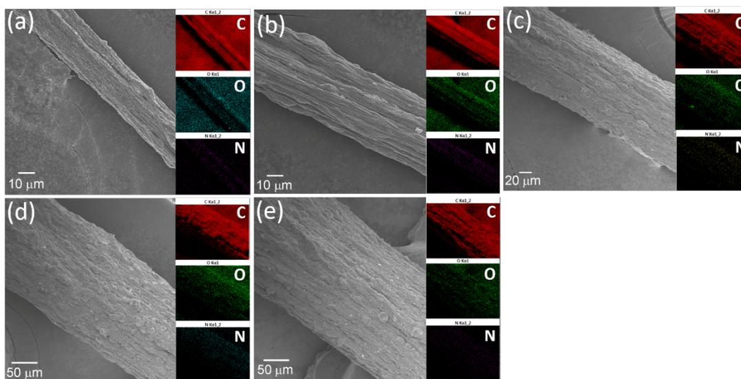
**Figure S4.** (a-e) SEM images of rGO/MWCNT hybrid fibers in different diameters with their EDX element (C, O and N) mappings in inserted images: (a) fiber-1, (b) fiber-2, (c) fiber-3, (d) fiber-4, and (e) fiber-5.
