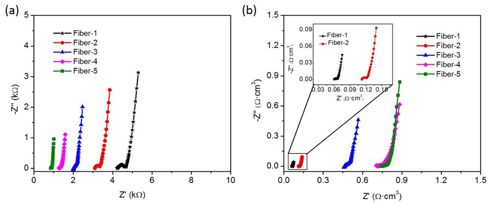
**Figure S11.** (a) Nyquist plot of hybrid carbon fibers in different diameters with frequency from 10 kHz to 0.01 Hz. (b) Nyquist plot normalized based on the volume of each fiber. The inset shows the enlarged normalized curves of fiber-1 and fiber-2.
