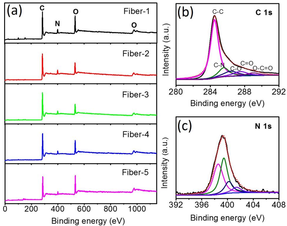
**Figure S5.** (a) XPS spectra of rGO/MWCNT hybrid fibers in different diameters. (b)  $C_{1s}$  spectrum and (c)  $N_{1s}$  spectrum of fiber-2.
