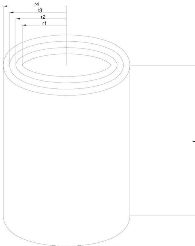
**Figure 1: Drawing of insulated solid storage tank for heat loss calculation**
