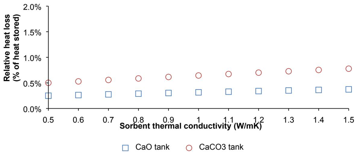
**Figure 6: Effect of sorbent thermal conductivity on the relative heat loss in the solid storage tank**
