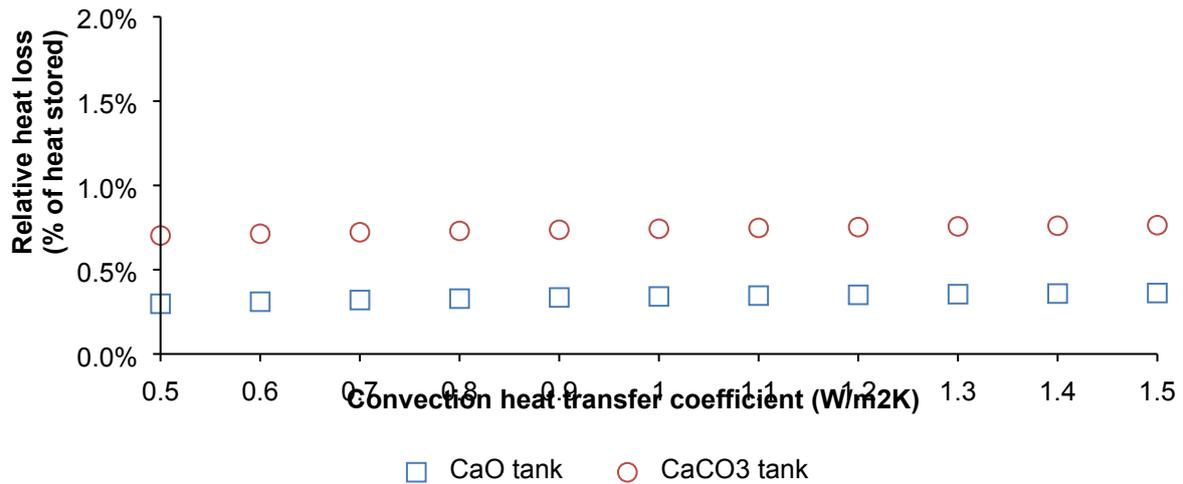
**Figure 7: Effect of convection heat transfer coefficient on the relative heat loss in the solid storage tank**
