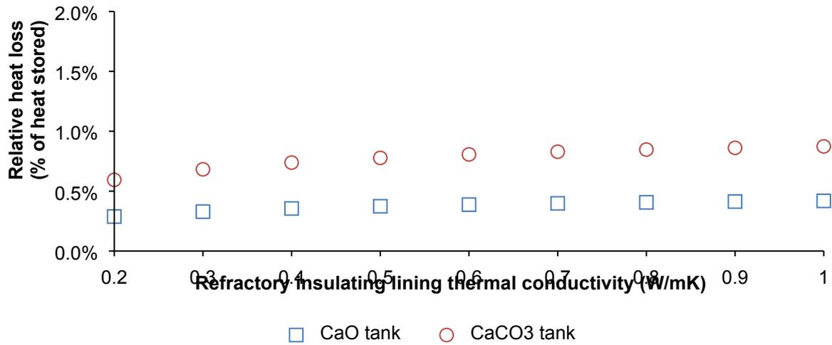
**Figure 5: Effect of refractory insulating lining thermal conductivity on the relative heat loss in the solid storage tank**
