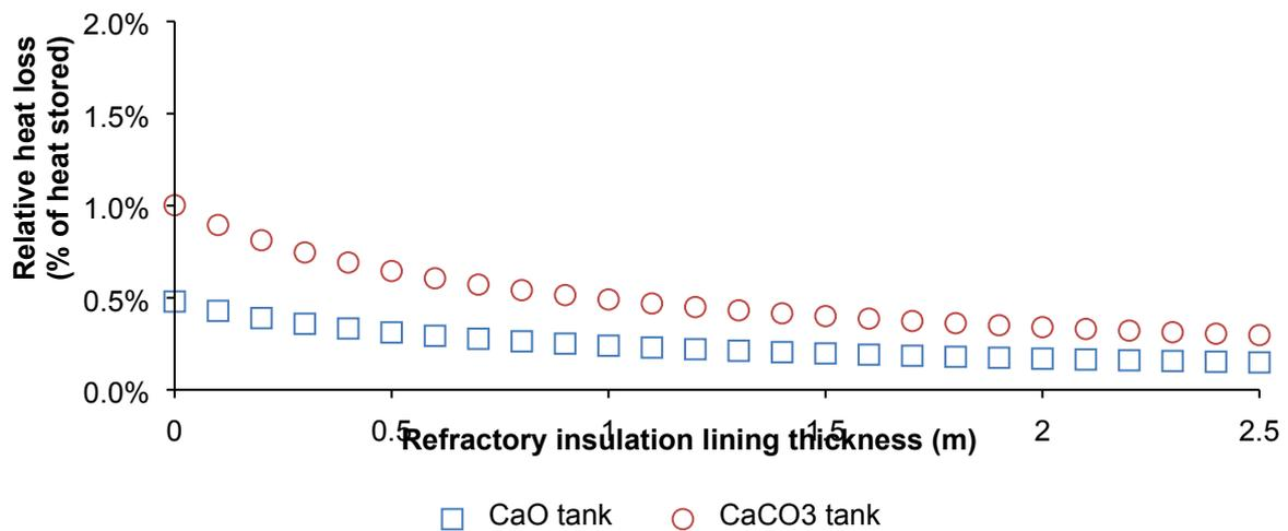
**Figure 3: Effect of the refractory insulation lining thickness on the relative heat loss in the solid storage tank**
