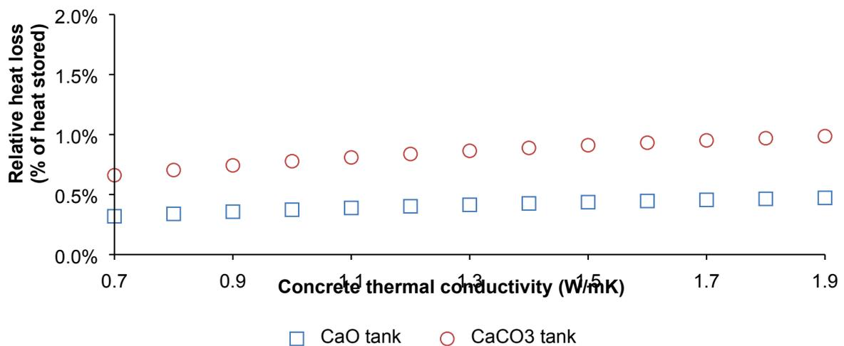
**Figure 4: Effect of concrete thermal conductivity on the relative heat loss in the solid storage tank**
