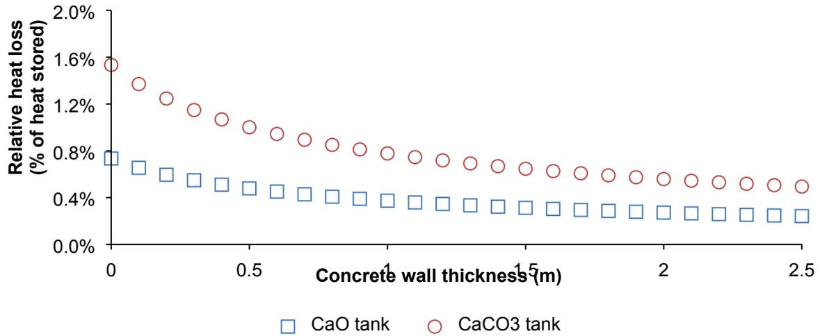
**Figure 2: Effect of the concrete wall thickness on the relative heat loss in the solid storage tank**
