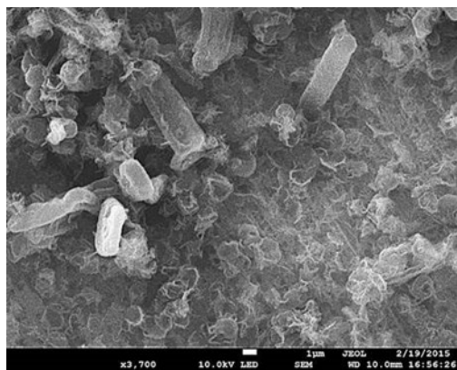
Figure S3. SEM image of lithium deposits on untreated copper current collector. Dendrites are visible.
