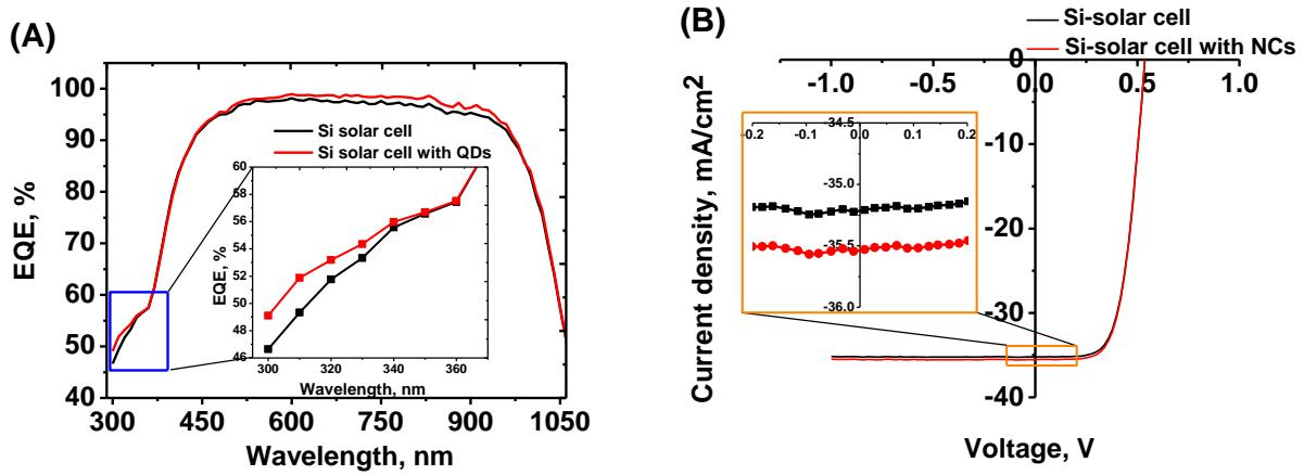
**Figure S6.** Panel A: Wavelength dependence of the external quantum efficiency (EQE) of a silicon solar cell coated with 1 mg/ml of  $Zn_{0.5}Cd_{0.5}S:Mn(5\%)/ZnS$  NCs dispersed in toluene. Panel B J–V curve of the same combination system.
