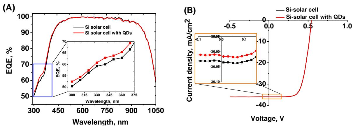
**Figure S9.** Panel A: Wavelength dependence of the external quantum efficiency (EQE) of a silicon solar cell coated with 15 mg/ml of  $Zn_{0.5}Cd_{0.5}S:Mn(5\%)/ZnS$  NCs dispersed in toluene; Panel B: J–V curve of the same system.
