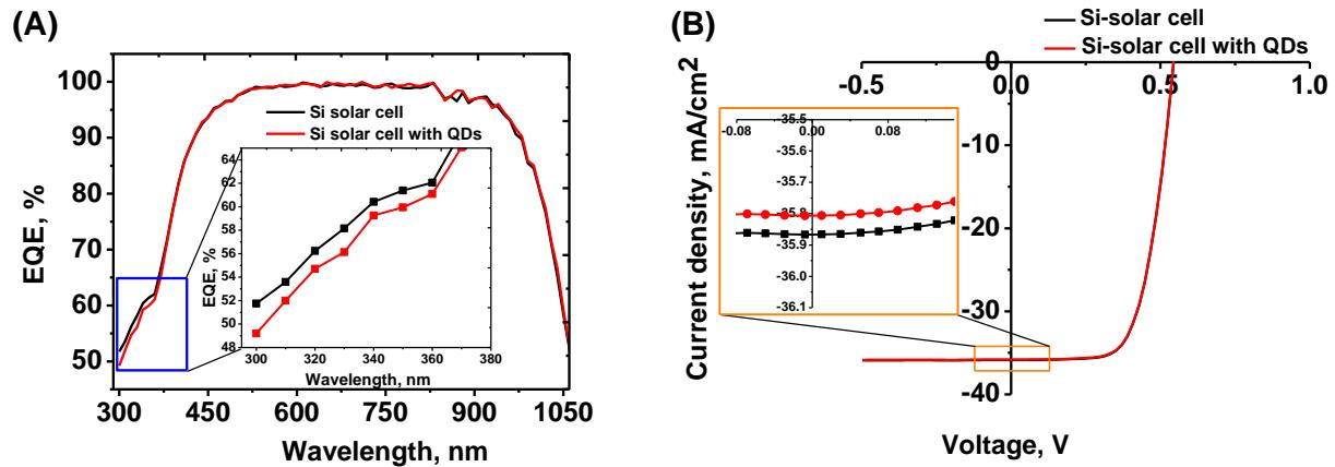
**Figure S10.** Panel A: Wavelength dependence of the external quantum efficiency (EQE) of a silicon solar cell coated with 20 mg/ml of  $Zn_{0.5}Cd_{0.5}S:Mn(5\%)/ZnS$  NCs dispersed in toluene; Panel B: J–V curve of the same system.
