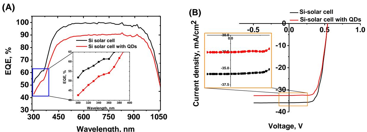
**Figure S11.** Panel A: Wavelength dependence of the external quantum efficiency (EQE) of a silicon solar cell coated with 25 mg/ml of  $Zn_{0.5}Cd_{0.5}S:Mn(5\%)/ZnS$  NCs dispersed in toluene; Panel B: J–V curve of the same system.
