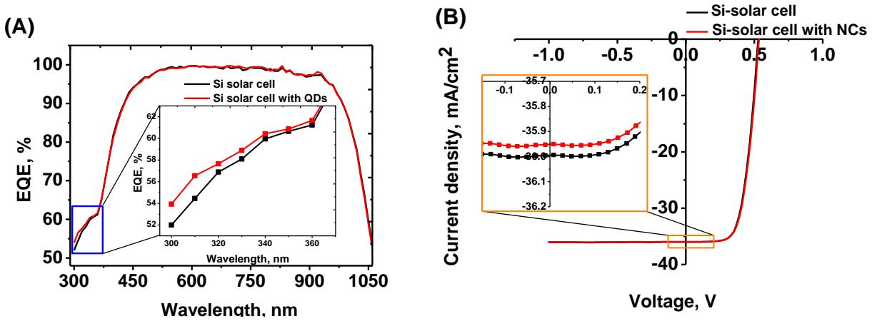
**Figure S5.** Panel A: Wavelength dependence of the external quantum efficiency (EQE) of a silicon solar cell coated with 0.5 mg/ml of  $Zn_{0.5}Cd_{0.5}S:Mn(5\%)/ZnS$  NCs dispersed in toluene. Panel B J–V curve of the same combination system.
