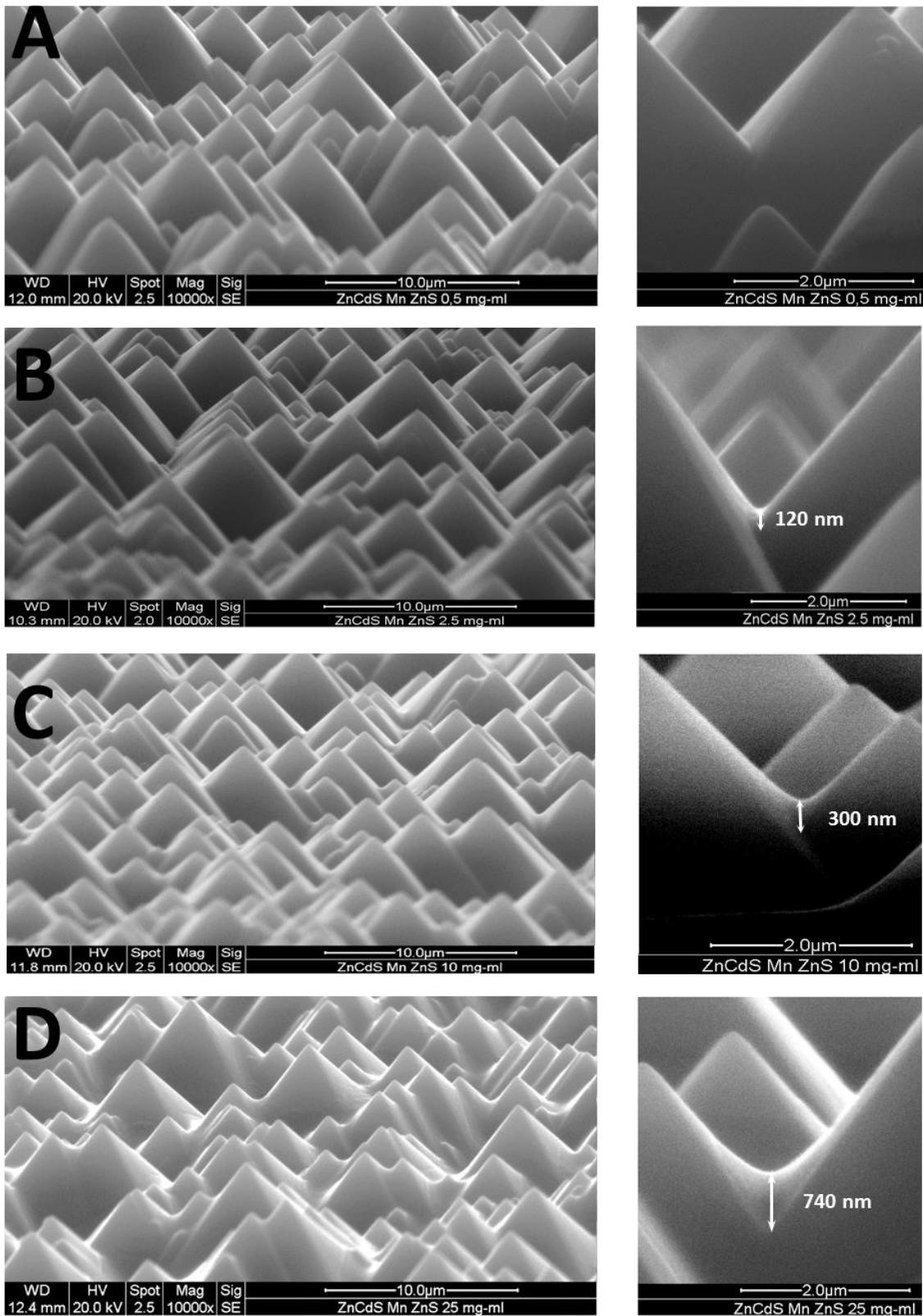
**Figure S12.** Selected SEM picture of the mono-Si solar cell surface structure cross-section of the same mono-Si solar coated with 0.5 mg/ml (a), 2.5 mg/ml (b), 5 mg/ml (c) and 25 mg/ml (d) NCs solution. The obtained NCs thicknesses varies from <50 to 750 nm.
