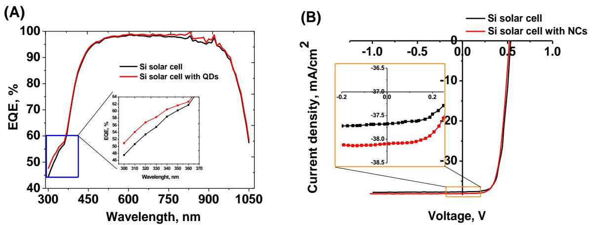
**Figure S7.** Panel A: Wavelength dependence of the external quantum efficiency (EQE) of a silicon solar cell coated with 2.5 mg/ml of  $Zn_{0.5}Cd_{0.5}S:Mn(5\%)/ZnS$  NCs dispersed in toluene. Panel B J–V curve of the same combination system.
