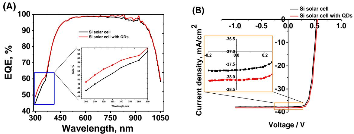
**Figure S8.** Panel A: Wavelength dependence of the external quantum efficiency (EQE) of a silicon solar cell coated with 5.0 mg/ml of  $Zn_{0.5}Cd_{0.5}S:Mn(5\%)/ZnS$  NCs dispersed in toluene; Panel B: J–V curve of the same system.
