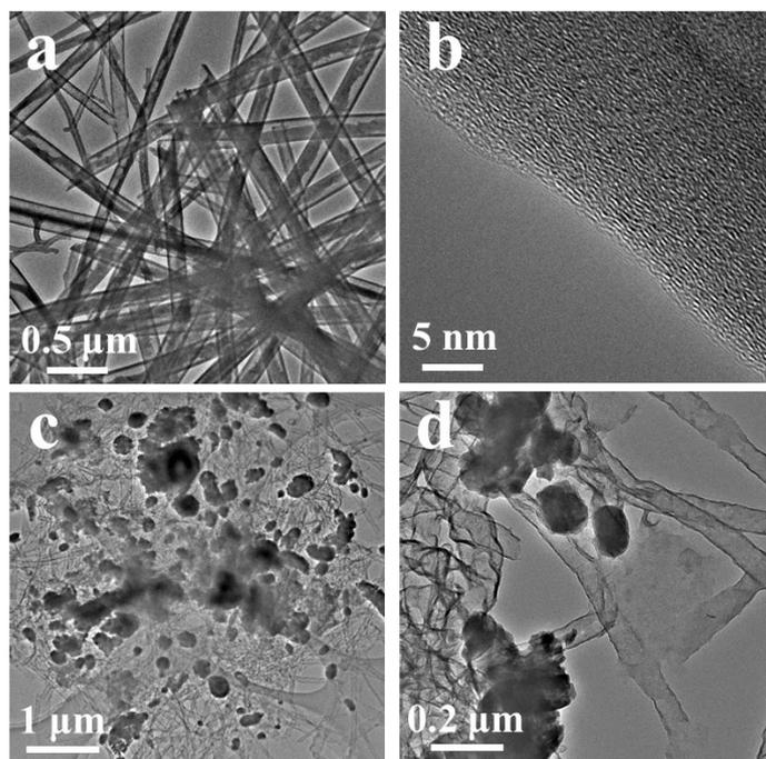
**Figure S8.** TEM images of  $V_2O_5@G$  after 100 cycles. (a) Scale bar, 500 nm. (b) Scale bar, 5 nm;
