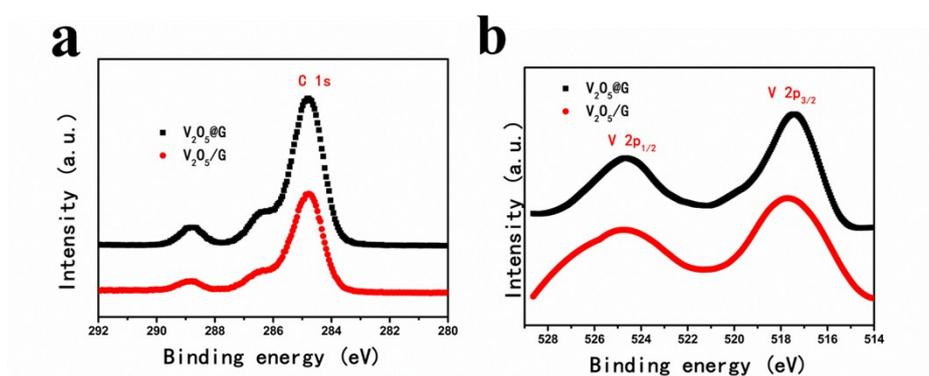
**Figure S5.** a) Survey XPS spectrum of  $V_2O_5@G$  and  $V_2O_5/G$ . (b) XPS spectrum of the V 2p
