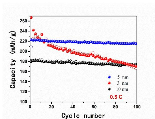
**Figure S7.** Different cycle performance of  $V_2O_5@G$  with different thickness of graphitic carbon coating via different CVD time (3.5 min, 5 min and 7 min respectively).
