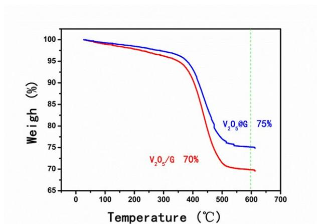
**Figure S6.** TGA of  $V_2O_5@G$  and  $V_2O_5/G$ . The TGA analysis was conducted in air using a heating rate of  $10\text{ }^\circ\text{C min}^{-1}$ . The weight loss from room temperature to  $200\text{ }^\circ\text{C}$  was mainly due to the removal of the physisorbed and chemisorbed water.
