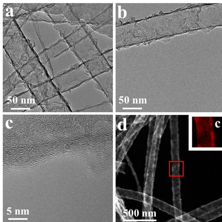
**Figure S9.** The TEM results of the sample after annealing to  $1070^{\circ}C$  without the presence of V source. (a) The TEM photos. scale bar, 50 nm; (b) The TEM photos. scale bar, 50 nm; (c) The
