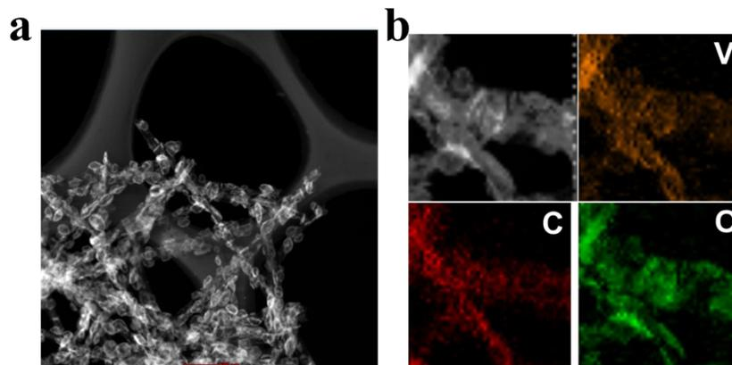
**Figure S4.** (a) Dark field transmission electron microscopy image of  $V_2O_5/G$ . Scale bar, 500 nm;
