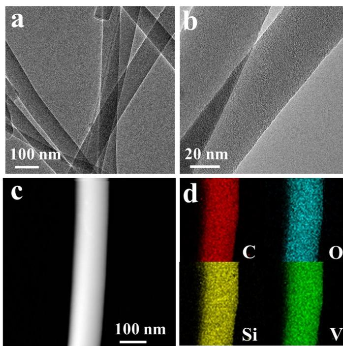
**Figure S3.** The TEM results of the sample after annealing to  $1070^\circ\text{C}$  without the presence of methane. (a) The TEM photos. scale bar, 100 nm; (b) The TEM photos. scale bar, 20 nm; (c) Dark field transmission electron microscopy image. Scale bar, 100 nm; (d) Carbon, Silicon, Oxygen and Vanadium elemental mapping of a selected area of an individual  $\text{V}_2\text{O}_5@\text{G}$ .
