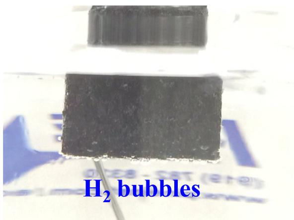
**Figure S20.** An optical image of EG/Co<sub>0.85</sub>Se/NiFe-LDH electrode during HER reaction; the bubbles indicate the formation of H<sub>2</sub> gas on EG/Co<sub>0.85</sub>Se/NiFe-LDH electrode.
