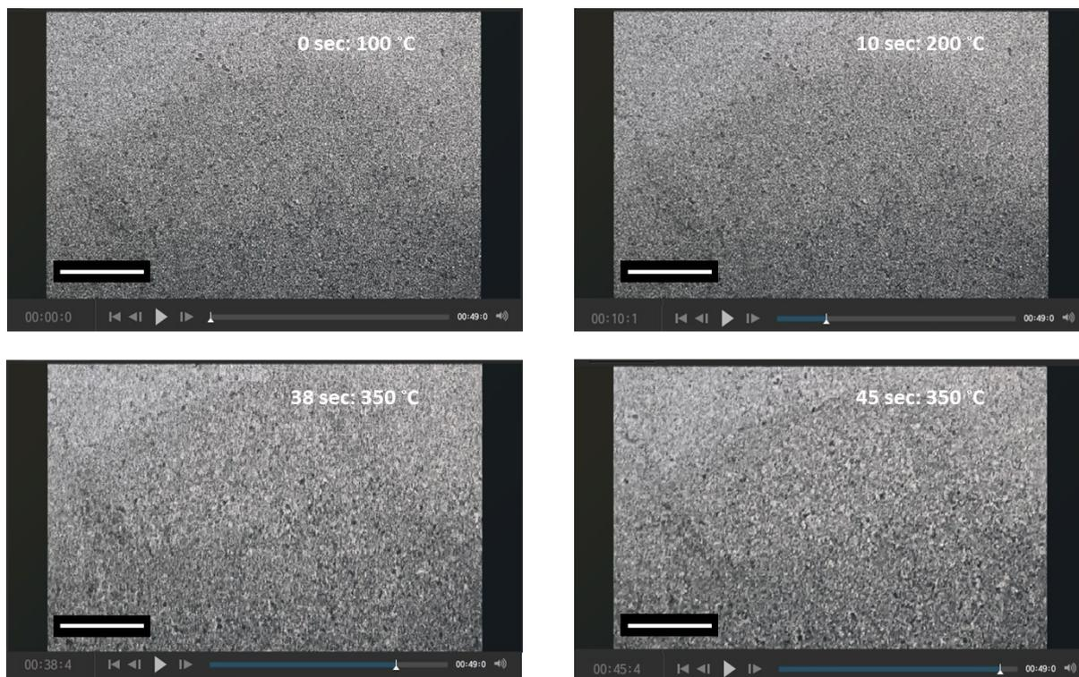
Snapshot in situ TEM images were recorded (x4) at 100–350 °C; at approximately 350 °C, SnO<sub>2</sub> on RGO induced carbon decomposition to introduce nanopores on the RGO sheets. Scale bars, 10 nm
