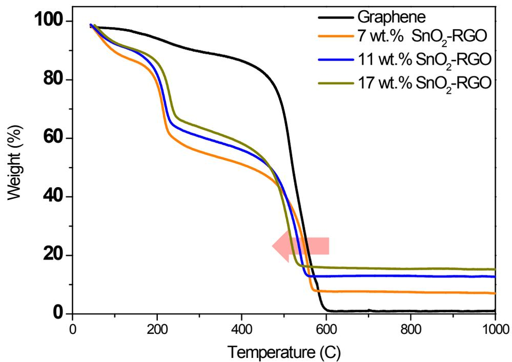
TGA profiles of P-graphene, 7wt.% SnO<sub>2</sub>-RGO, 11wt.% SnO<sub>2</sub>-RGO, and 17wt.% SnO<sub>2</sub>-RGO. The catalytic carbon decomposition temperature decreased with increasing amounts of SnO<sub>2</sub>.
