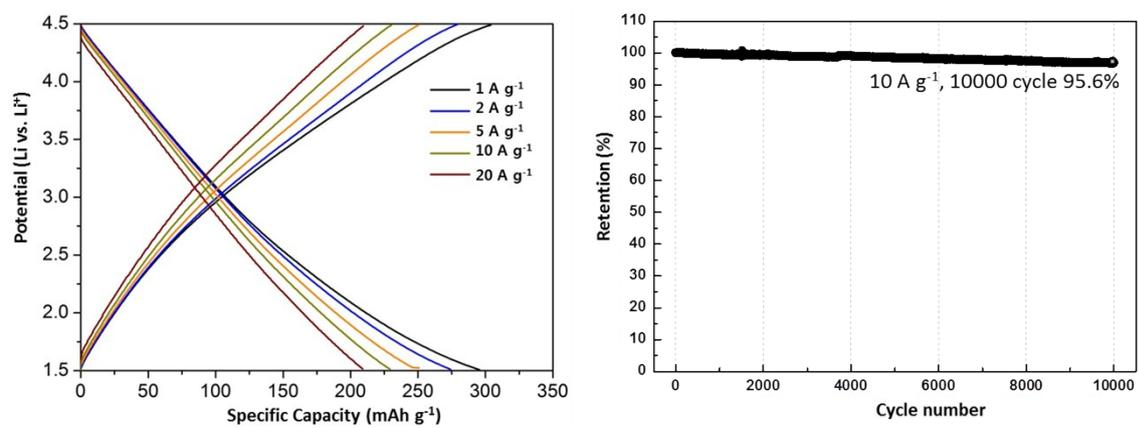
Electrochemical properties of GNM electrodes in the three-electrode test using 1 M LiPF<sub>6</sub> in EC/DMC (1:1 v/v).
