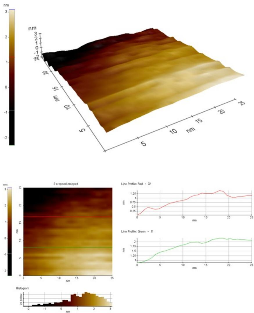
AFM image and height profile of P-graphene.
