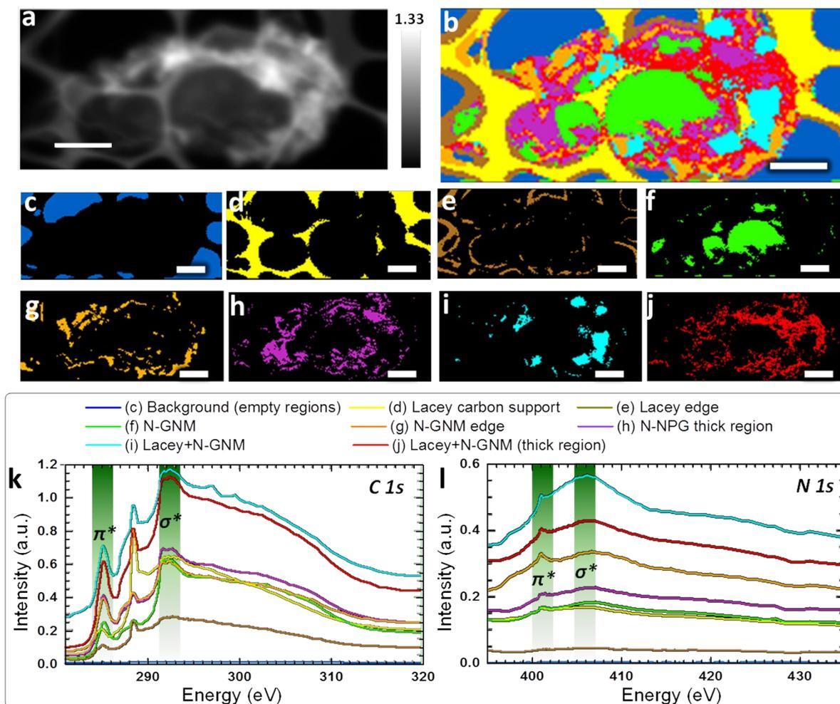
(a) The overall morphology of a selected single N-GNM sheet; the vertical gray scale represents the optical density. (Scale bar, 1 μm) (b) The color composite map was generated from the average OD image by combining individual component maps (Scale bar, 1 μm) (c-j) using principal component analysis; the corresponding. (Scale bars, 1 μm) (k) C and (l) N K-edge NEXAFS spectra were derived from the same regions.
