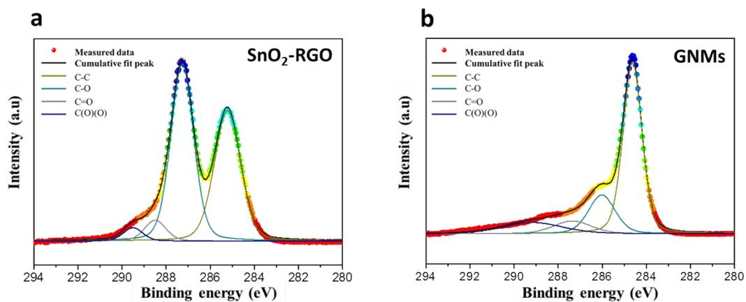
C 1s XPS spectra of (a) SnO<sub>2</sub>-RGO and (b) GNMs. The O/C ratio of SnO<sub>2</sub>-RGO decreases remarkably during the preparation of GNMs, indicating the successful removal of most of the epoxide and hydroxyl functional groups.
