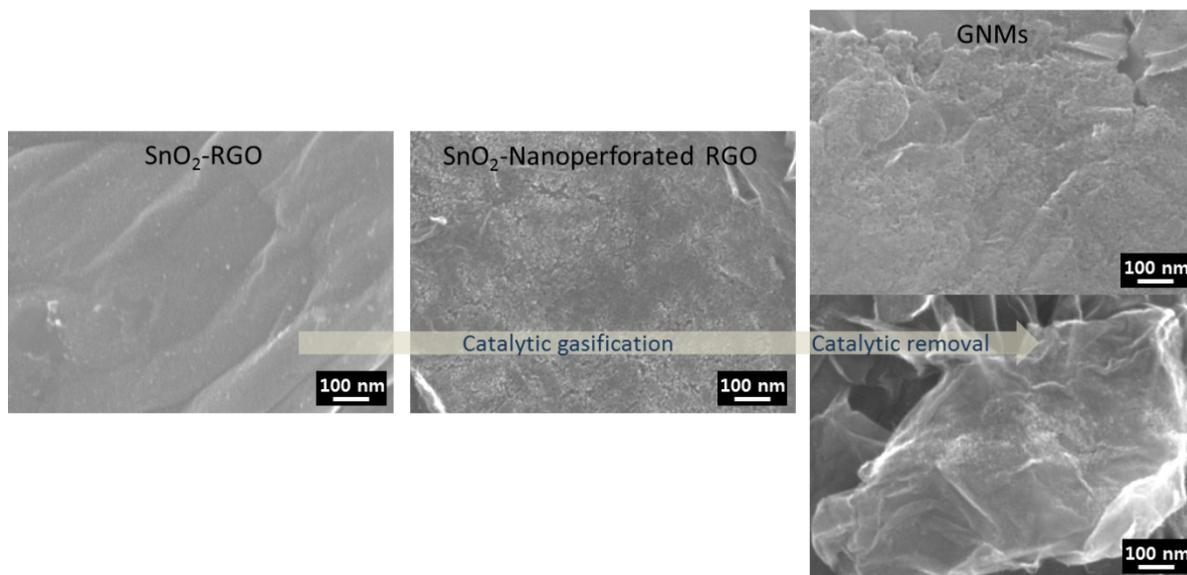
SEM images of SnO<sub>2</sub>-RGO, SnO<sub>2</sub>-nanoperforated RGO via carbon catalytic gasification, and GNMs
