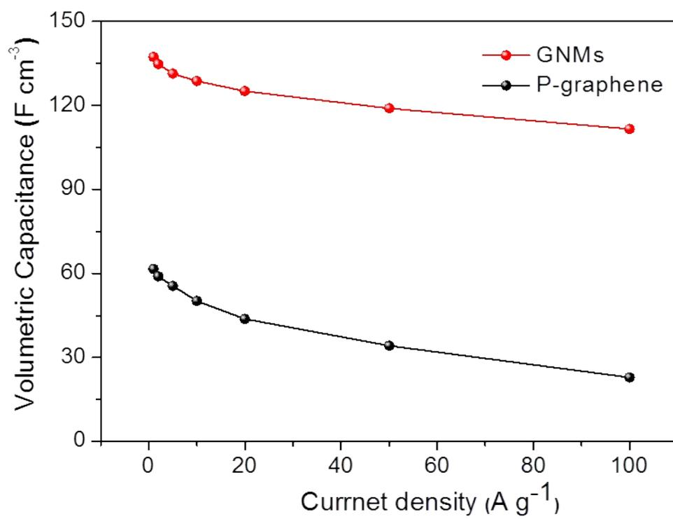
Volumetric capacitance of GNMs (packing density: 0.54 g cm<sup>-1</sup>) and P-graphene (packing density: 0.38 g cm<sup>-1</sup>) electrodes.
