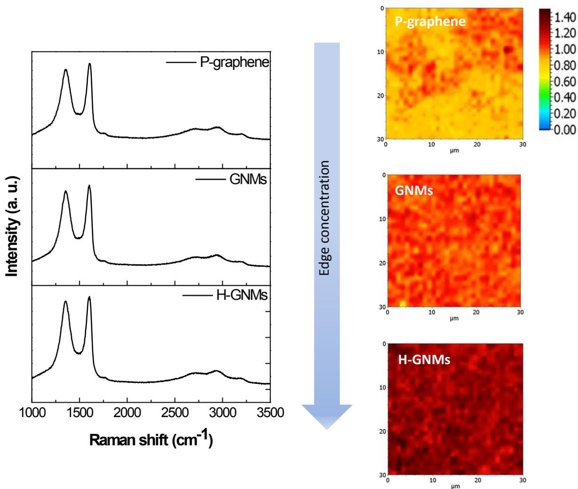
Raman spectra and mapping images ( $30 \mu\text{m} \times 30 \mu\text{m}$ ) of P-graphene, GNMs, and H-GNMs. The differences in D/G ratio of P-graphene and NPG are clearly observed by color differences.
