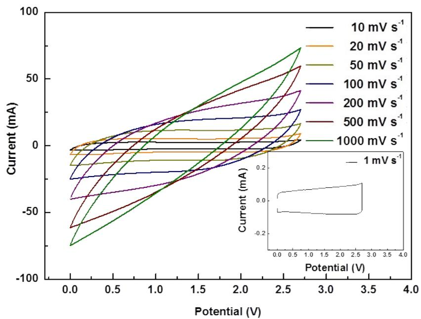
Cyclic voltammogram for P-graphene. Compared with GNMs, P-graphene shows poor cyclic voltammetric behaviors.
