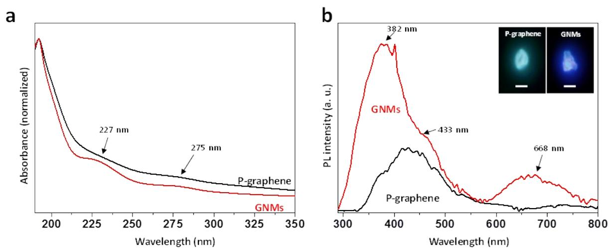
(a) UV-vis absorption and fluorescence spectra and (b) PL spectra of P-graphene and GNM (0.01 mg/ml in ethanol/H<sub>2</sub>O (1/1 v/v ratio)) Inset: digital images indicate blue and green PL emissions of P-graphene and GNM. Scale bar, 20 μm.
