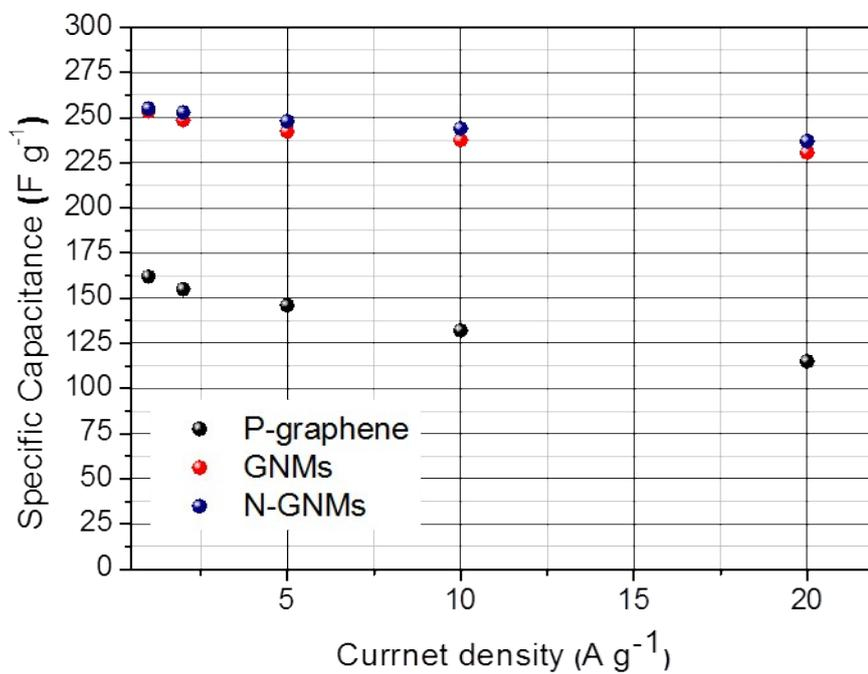
Rate capabilities of P-graphene, GNMs and N-GNMs at various current densities between 1 and 20 A g<sup>-1</sup>. The N-GNMs (specific capacitances of 255, 252, 248, 244 and 236 F g<sup>-1</sup> at current densities of 1, 2, 5, 10 and 20 A g<sup>-1</sup>) exhibit slightly enhanced specific capacitance and rate capability than GNMs electrode.
