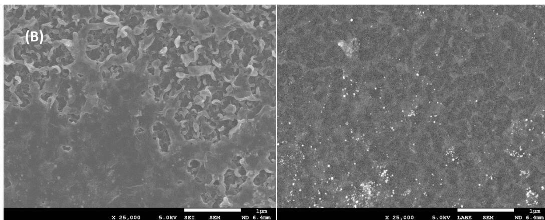
51 FIGURE S1. FE-SEM images and backscatter electron imaging for (A) GO functionalized TFC,
