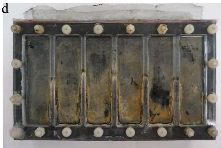
Figure S2. (a) Photograph of cathode cassette with mesh spacers, (b) schematic showing dimensions of the column spacer, (c) the position of washers in the wire spacers, and (d) the dilute hydrochloric acid cleaned cathode module after wastewater operation.
