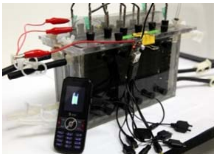
Figure S9. Photographs of the MFC module fed domestic wastewater that was used to power a fan or charge an AT&T cellphone.
