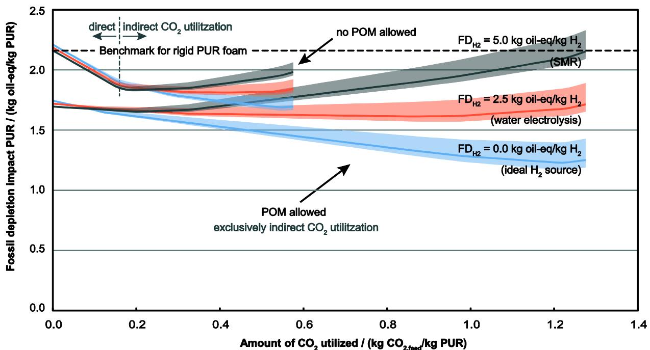
**Figure S 3** Minimum fossil depletion for rigid PUR foams for variable amounts of CO<sub>2</sub> utilized. The transparent areas indicate the range for alternative CO<sub>2</sub> sources: lower bounds correspond to an ideal source, upper bounds correspond to CO<sub>2</sub> capture from ambient air, and the solid lines correspond to CO<sub>2</sub> capture from a coal-fired power plant.
