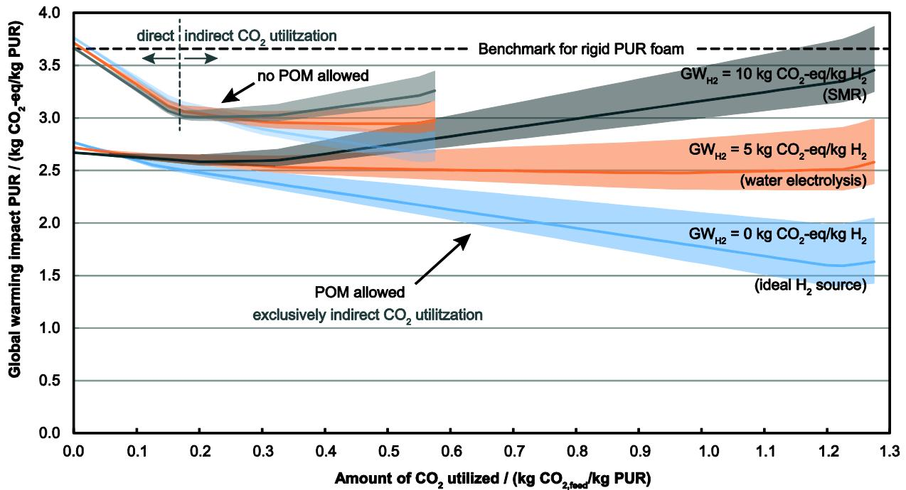
**Figure S 2** Minimum global warming impact for rigid PUR foams for variable amounts of CO<sub>2</sub> utilized. The transparent areas indicate the range for alternative CO<sub>2</sub> sources: lower bounds correspond to an ideal source, upper bounds correspond to CO<sub>2</sub> capture from ambient air, and the solid lines correspond to CO<sub>2</sub> capture from a coal-fired power plant.
