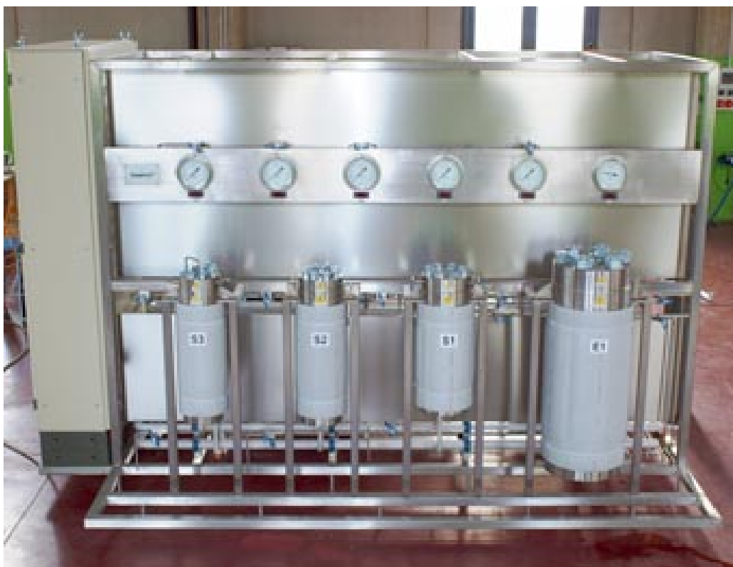
Figure S1. Supercritical CO 2 extraction pilot scale plant used for the experimental work: SFE100 Series Plant – Separeco Srl, Italy
