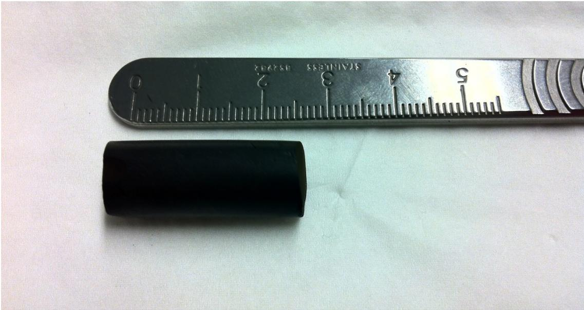
Fig. S 8 Monolith of Starbon® after carbonisation at 800 °C.
