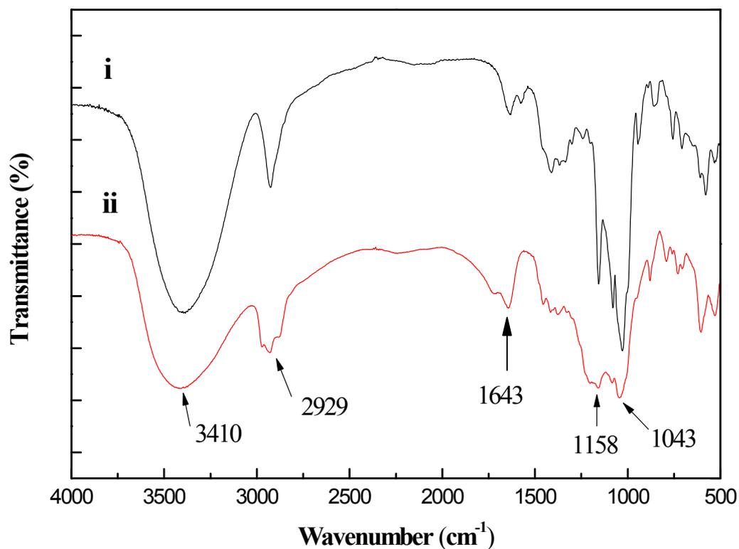
Fig. S1 FT-IR spectra of  $\beta$ -CD and  $\beta$ -CD-BSA in KBr
