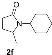
**5-methyl-N-cyclohexylpyrrolidone (5MeNcHP) 2f** was synthesized following the procedure B on 60 mmol scale. Volume of reactor 200mL, temperature 140°C. Maximum pressure set to 23 bar, measured 20 bar after 8h. Conversion 89 %. Isolated by distillation as a yellowish colorless oil. Yield 88 %.
