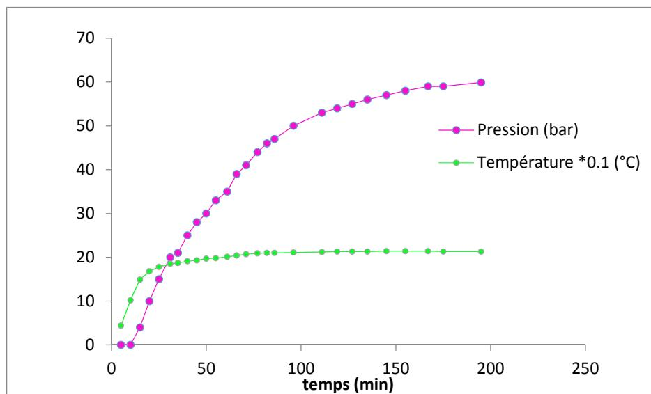
Conditions : Conditions: LA (120 mmol), propylamine (120 mmol), HCOOH (120 mmol), in 100mL autoclave. Set temperature 200°C, maximum pressure set 64 bars, measured 62 bars.
