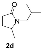
**5-methyl-N-isobutylpyrrolidone (5MeNiBP) 2d** was synthesized following the procedure A1 and isolated as colorless liquid with 87% yield. **2d** was synthesized following the procedure B on 110 mmol scale. Volume of reactor 200mL, temperature 160°C, maximum pressure set 22 bar, measured 22 bar after 6.8h. Conversion > 99 %. Isolated by distillation as a colorless oil. Yield 86%.
