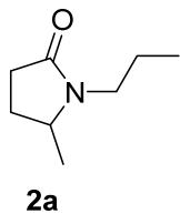
**5-methyl-N-propylpyrrolidone (5MeNPP) 2a** was synthesized following the procedure A1 and isolated as colorless liquid with 64% yield. **2a** was synthesized following the procedure B on 60 mmol scale. Volume of reactor 100mL, temperature 160°C, maximum pressure set 25 bars, measured 25 bar after 4.2 h. Conversion > 99 %. Isolated by distillation as a colorless oil. Yield 84 %. See the Temperature and Pressure chart above.
