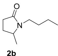
**5-methyl-N-butylpyrrolidone (5MeNBP) 2b** was synthesized following the procedure A1 and isolated as colorless liquid with 49% yield. **2b** was synthesized following the procedure B on 120 mmol scale. Volume of reactor 200 mL, temperature 200°C. Maximum pressure set 26 bar, measured 26 bar. Conversion > 99 %. Isolated by distillation as a colorless oil. Yield 82 %.
