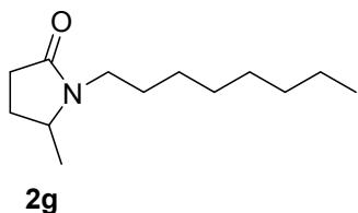
**5-methyl-N-n-octylpyrrolidone** (MeNOP) **2g** was synthesized following the procedures A1 and A2 and isolated as an orange oil with 80% yield. **2g** was also synthesized following the procedure B on 120 mmol scale. Volume of reactor 200mL, temperature 180°C, maximum pressure set 28 bar, measured 24 bar. Conversion 86 %. Isolated by extraction as yellow oil. Yield 80%.
