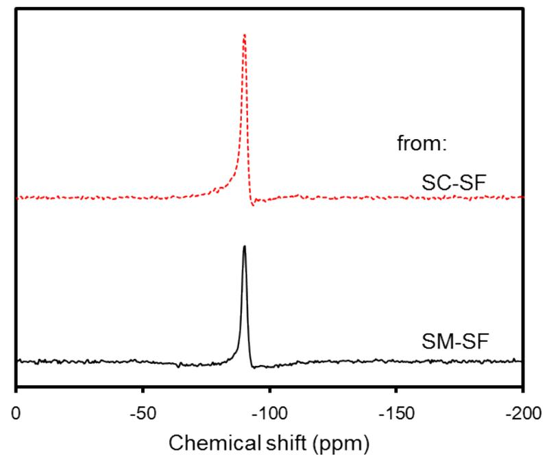
Fig. S1.  $^{29}\text{Si}$  MAS NMR spectra of zeolite A synthesized from SM-SF (solid line) and SC-SF (dotted line) at 70 °C for 5 h.
