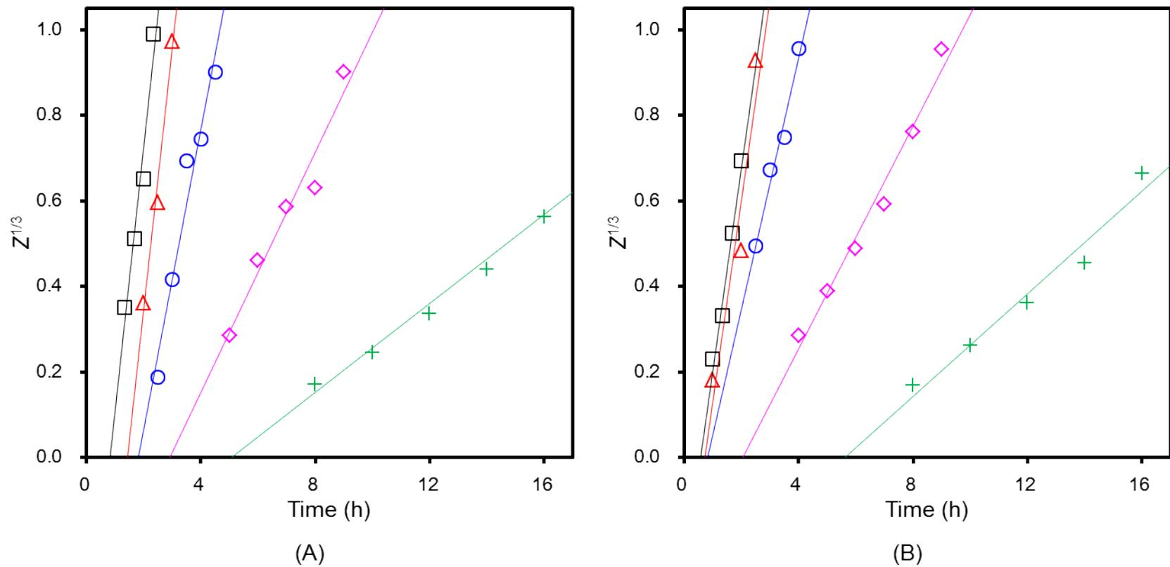
Fig. S4. Plot of  $Z^{1/3}$  vs time in the crystallization of zeolite A from (A) SM-SF and (B) SC-SF at different temperatures: (+) 50 °C, ( $\diamond$ ) 60 °C, ( $\circ$ ) 70 °C, ( $\Delta$ ) 80 °C and ( $\square$ ) 90 °C.
