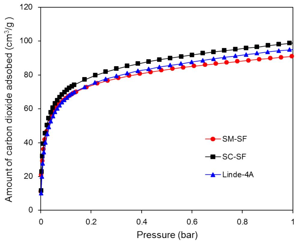
Fig. S3. Adsorption isotherms of carbon dioxide on LTA zeolites at 273 K.
