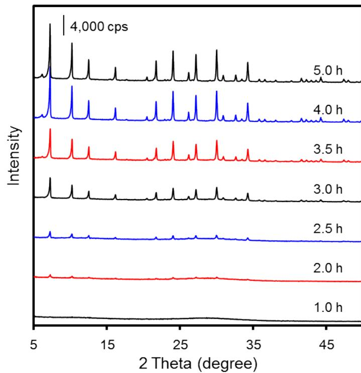
Fig. S7. XRD patterns of solid phases obtained in the crystallization of zeolite A from SC-FF1 at 70 °C
