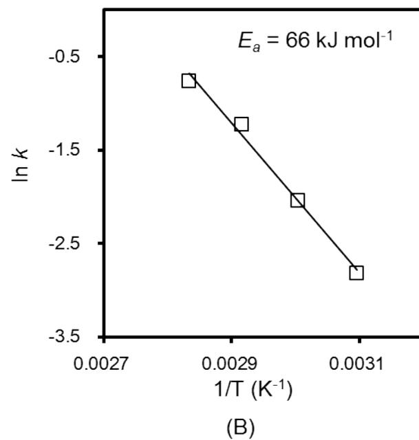
Fig. S5. Arrhenius plots for the crystallization of zeolite A from (A) SM-SF and (B) SC-SF.
