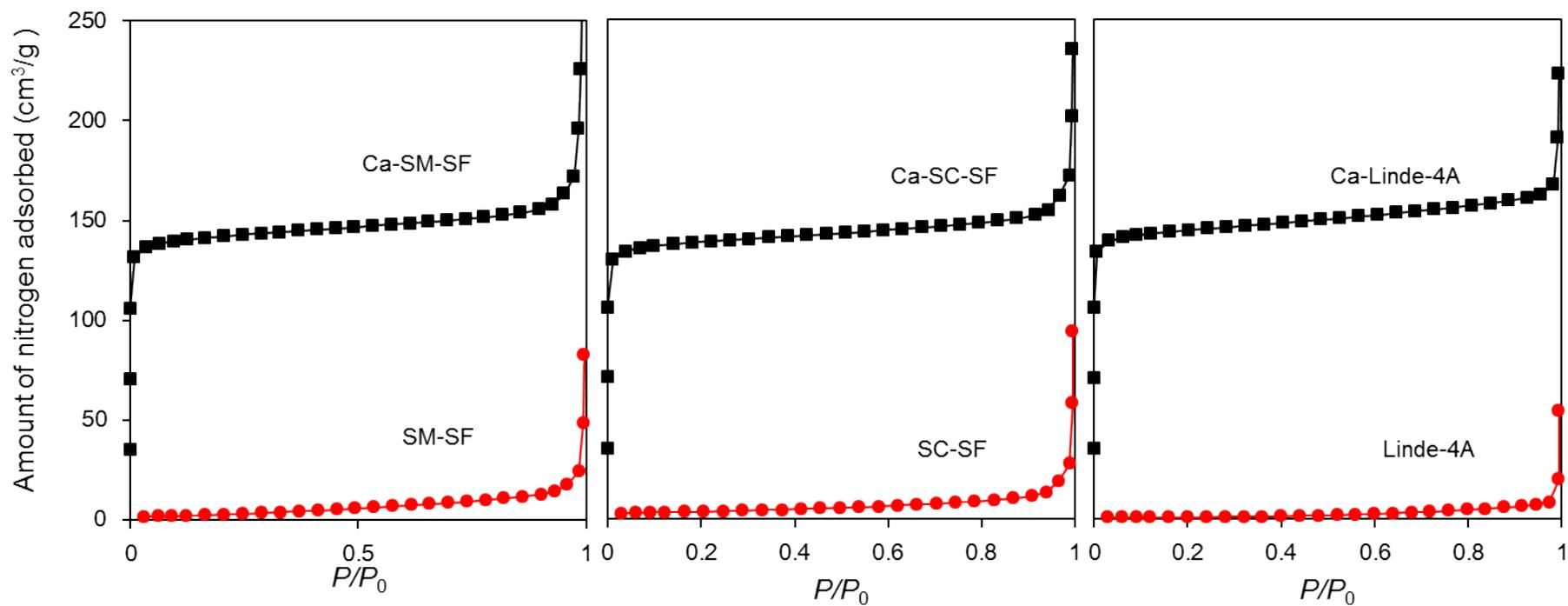
Fig. S2. Adsorption isotherms of nitrogen on LTA zeolites (A) SM-SF, (B) SC-SF, and (C) Linde-4A at 77 K. Calcium ion-exchanged LTA zeolites were denoted by adding “Ca” in front of their names.
