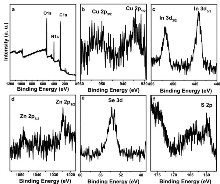
**Figure S6** XPS analysis of the CISE/ZnS (Cu/In=1/8) core/shell QDs. (a) the survey-scan XPS picture and narrow-scan of the Cu 2p region (b), In 3d region (c), Zn 2p region (d), Se 3d region (e) and S 2p region (f).
