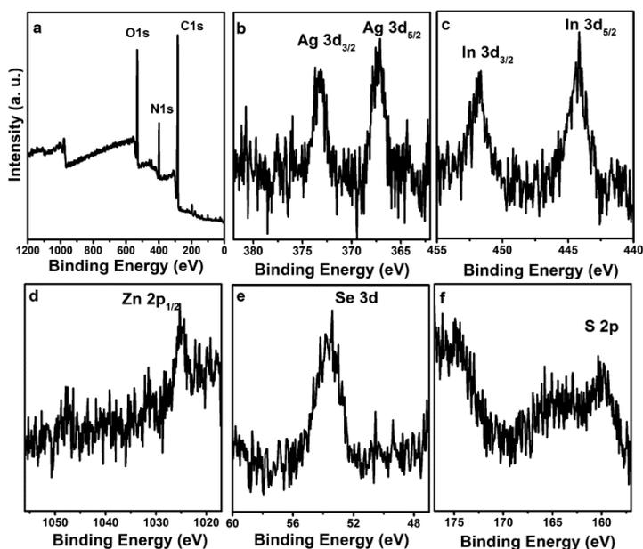
**Figure S7** XPS analysis of the AISE/ZnS (Ag/In=1/8) core/shell QDs. (a) the survey-scan XPS picture and narrow-scan of the Ag 3d region (b), In 3d region (c), Zn 2p region (d), Se 3d region (e) and S 2p region (f).
