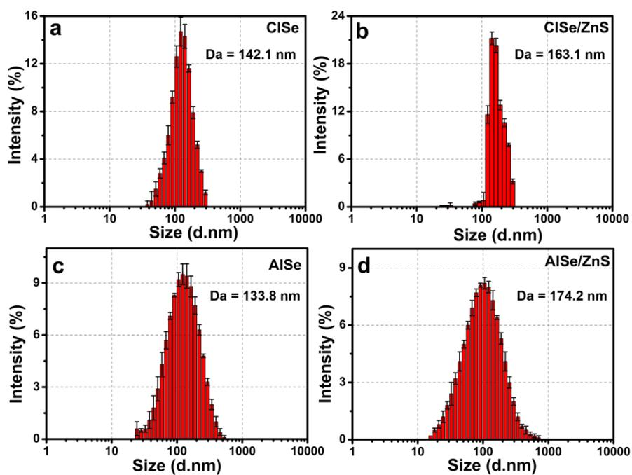
**Figure S4** Particle size distributions of CISE cores (Cu/In=1/8) (a), the corresponding CISE/ZnS core/shell QDs (b), AISE cores (Ag/In=1/8) (c) and the corresponding AISE/ZnS core/shell QDs (d) in water, determined by dynamic light scattering (DLS).
