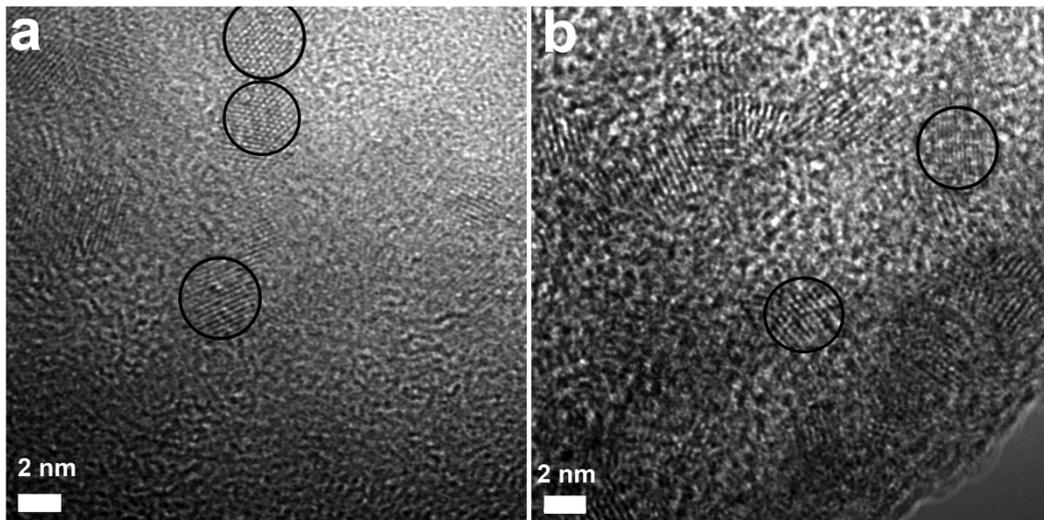
**Figure S3** HRTEM images of CISE/ZnS (Cu/In=1/8) (a) and AISe/ZnS (Ag/In=1/8) (b) core/shell QDs.
