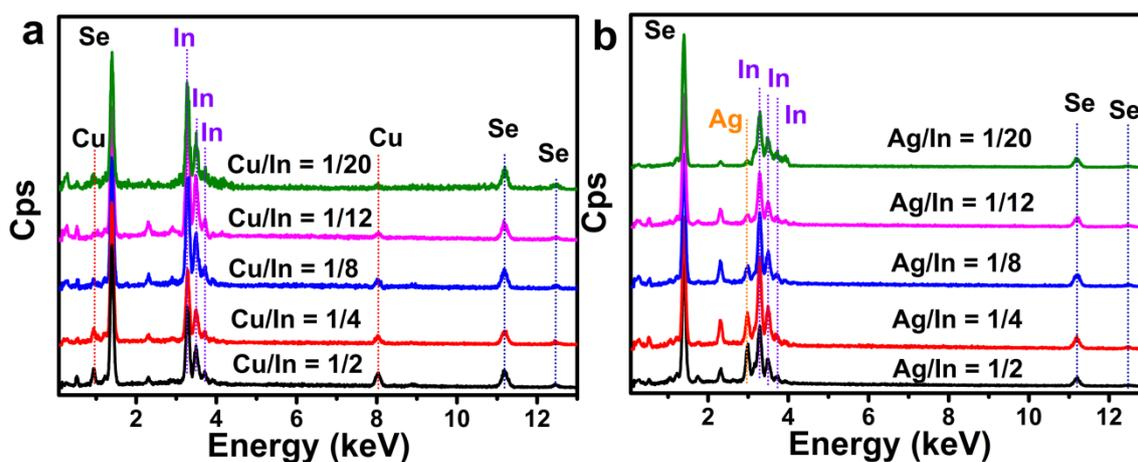
**Figure S5** EDS spectra of CISE core QDs and AISE core QDs with different precursor ratios.
