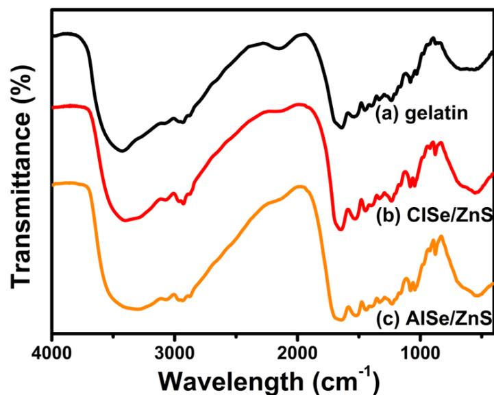
**Figure S8** FT-IR spectra of pure gelatin (a), CISe/ZnS (b) and AISe/ZnS (c) core/shell QDs.
