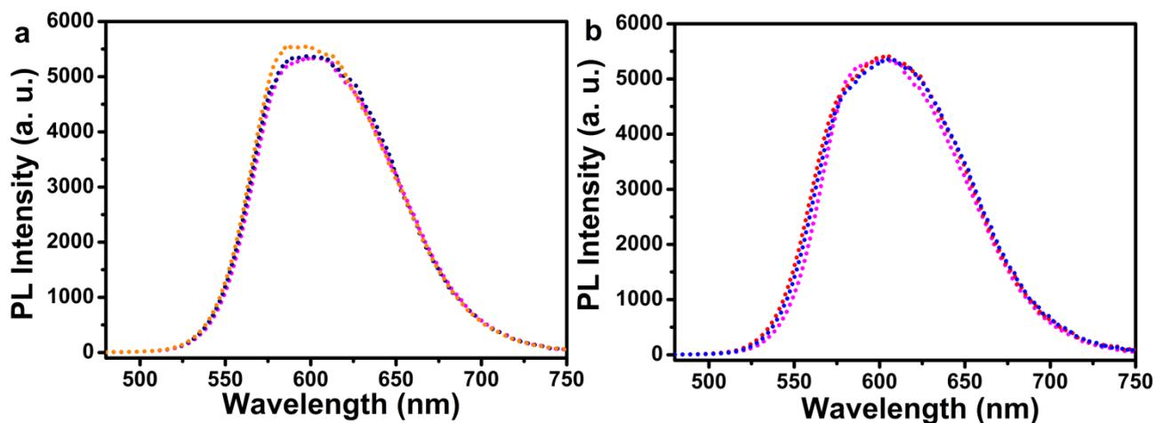
**Figure S1.** PL spectra of AgInSe<sub>2</sub>/ZnS (Ag/In = 1/12) core/shell QDs synthesized in different electric pressure cookers (a) and in different batches which are synthesized in the same electric pressure cooker (b).
