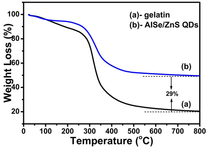
**Figure S2.** TG curves of pure gelatin (a) and AISe/ZnS (Ag/In=1/12) core/shell QDs (b).
