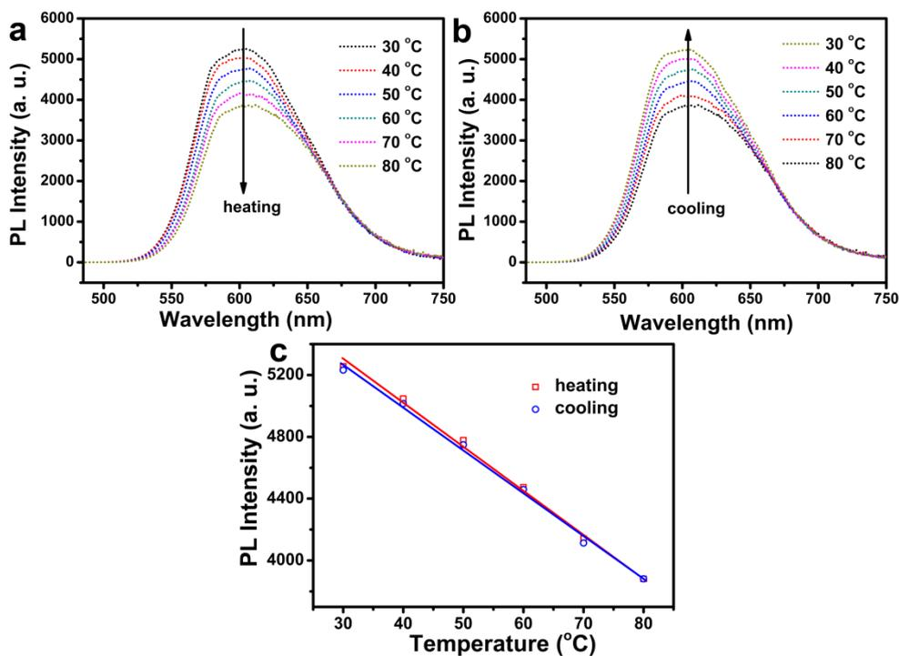
**Figure S9** Temperature-dependent PL spectra of AISe/ZnS (Ag/In = 1/12) core/shell QDs in a heating (a)-cooling (b) cycle; (c) PL intensity shifts of AISe/ZnS core/shell QDs over temperature.
