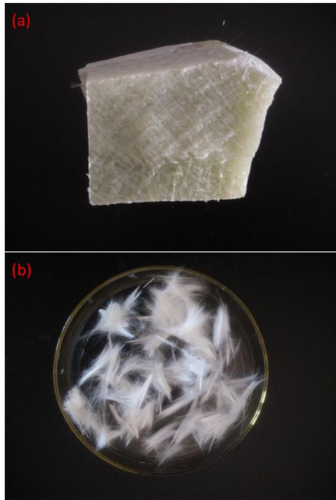
**SI Figure 18.** Recycled glass fibres from GFRP. Degradation condition: 10 wt%  $\text{AlCl}_3/\text{CH}_3\text{COOH}$ , 180 °C, 9 h. (a) GFRP, (b) recycled glass fiber.
