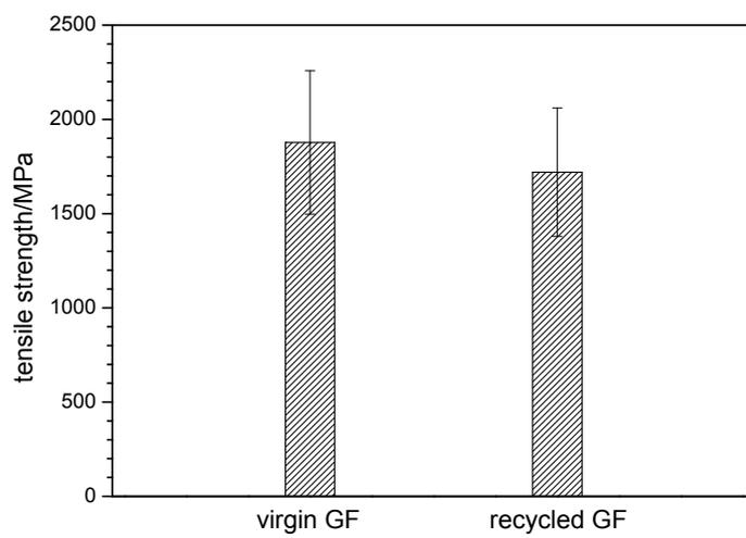
**SI Figure 19.** Monofilament tensile strength of virgin GF and recycled GF. Degradation condition: 10 wt%  $\text{AlCl}_3/\text{CH}_3\text{COOH}$ , 180 °C, 9 h.
