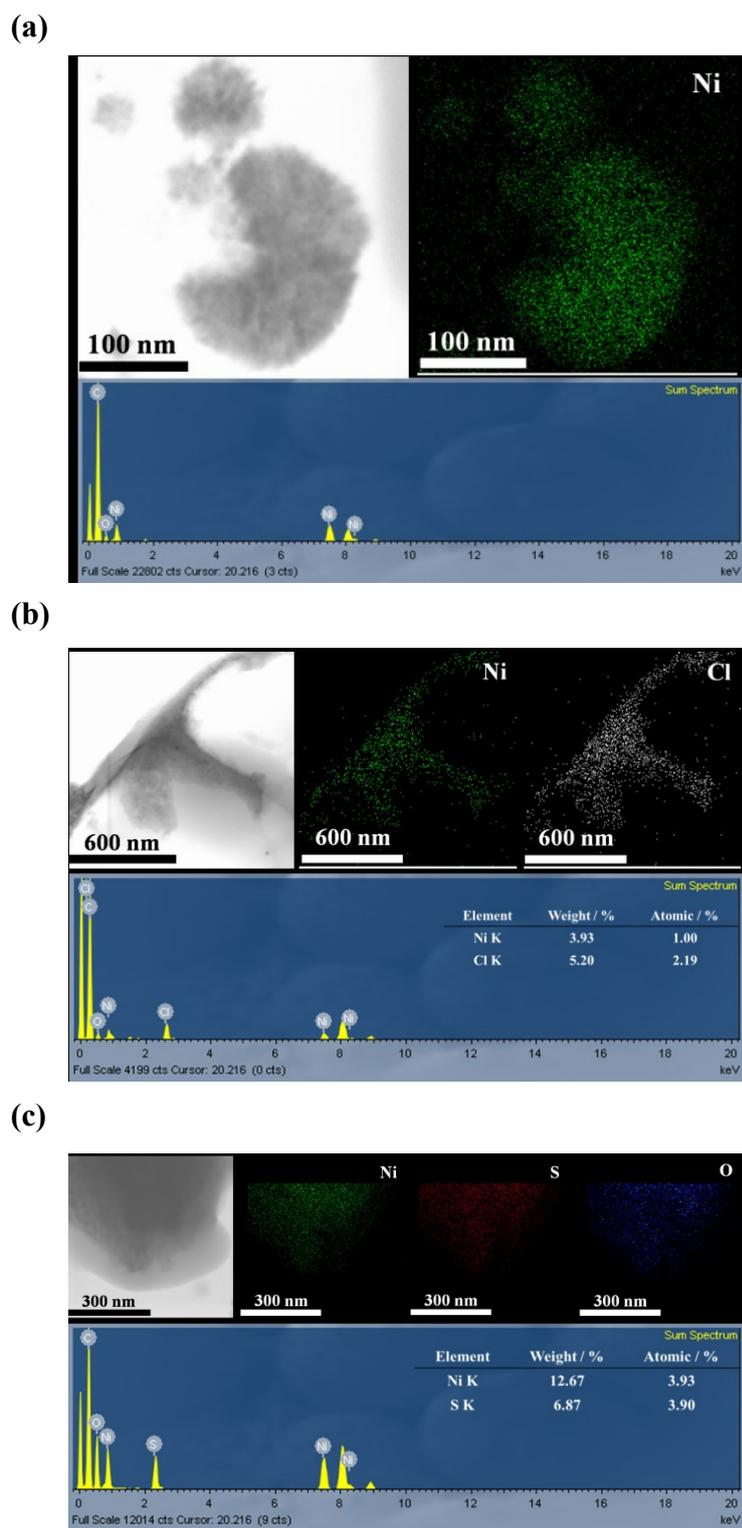
**Fig. S4** TEM images and element mapping of different nickel salts after reaction with stearic acid. (a)  $\text{Ni}(\text{OAc})_2$ ; (b)  $\text{NiCl}_2$ ; (c)  $\text{NiSO}_4$ .
