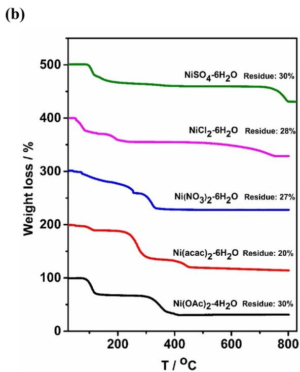
**Fig. S1** Thermogravimetric analysis under N<sub>2</sub> flow. (a) different acetate salts; (b) different nickel salts.
