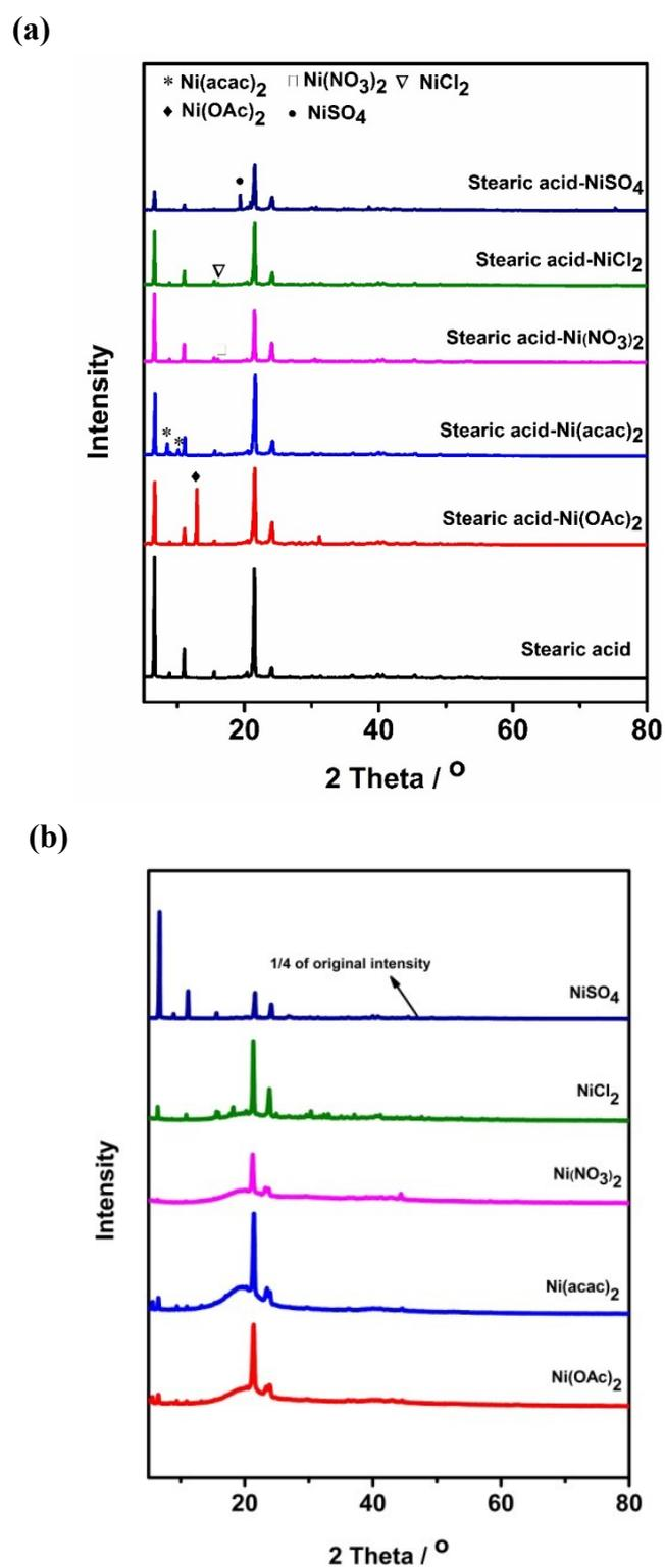
**Fig. S2** XRD patterns of different nickel salts with stearic acid. (a) before reaction; (b) after reaction.
