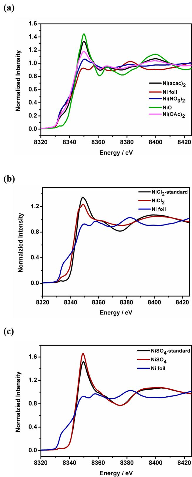
**Fig. S3** XAS spectra of different nickel slats. (a)  $\text{Ni}(\text{OAc})_2$ ,  $\text{Ni}(\text{acac})_2$  and  $\text{Ni}(\text{NO}_3)_2$  catalytic systems; (b)  $\text{NiCl}_2$  catalytic system; (c)  $\text{NiSO}_4$  catalytic system.
