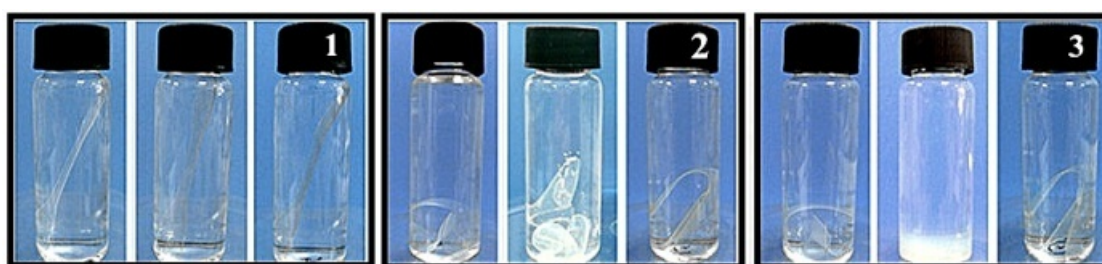
Fig .6a The alkaline resistance of various WPU, the photos of group 1, 2, 3 correspond to the beginning of immersing, after 300 min and 520 min immersion, respectively. In each group, the left, middle, and right photos correspond to CO 2 -WPU, PBA-WPU and PPG-WPU, respectively.
