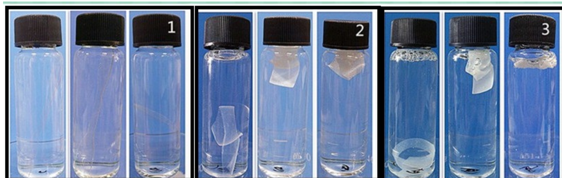
Fig .6d The oxidation resistance of various WPU, the photos of group 1, 2, 3 correspond to the beginning of immersing, after 5 h and 20 h immersion, respectively. In each group, the left, middle, and right photos correspond to CO 2 -WPU, PBA-WPU and PPG-WPU, respectively.
