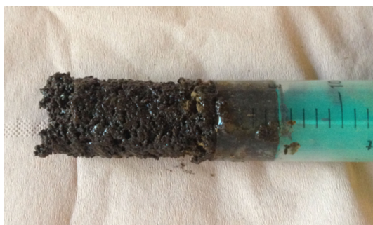
Figure S11. Attempts to make lignin-silicone foams using DMS-H41 (F-12) failed due to the high intrinsic viscosity of DMS-H41. The precursor is semi-cured, and could not be processed in extruder.
