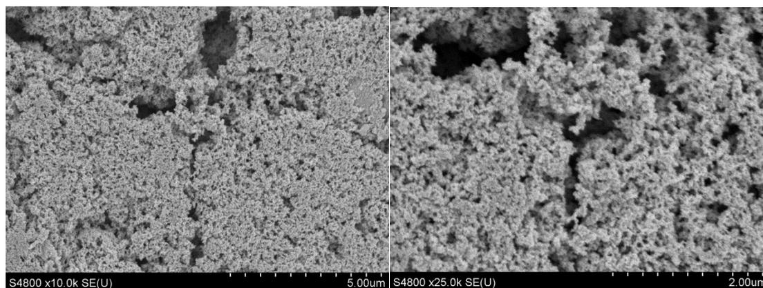
**Fig. S8** FE-SEM patterns of [PYD]@Pd after used for 15 times with different magnification, left (10k), right (25k).
