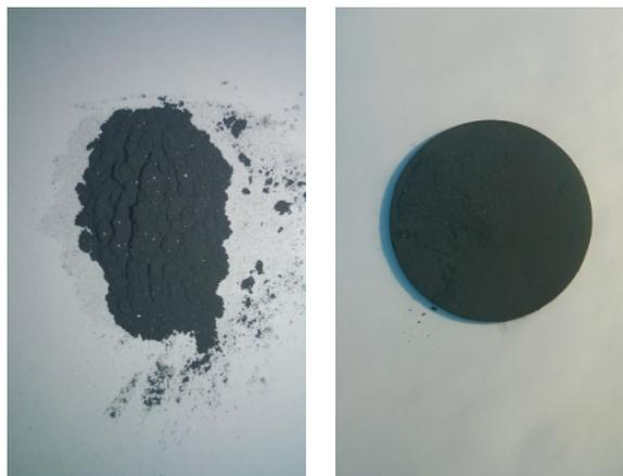
**Fig. S3** [PYD]@Pd before (left) and after (right) press.
