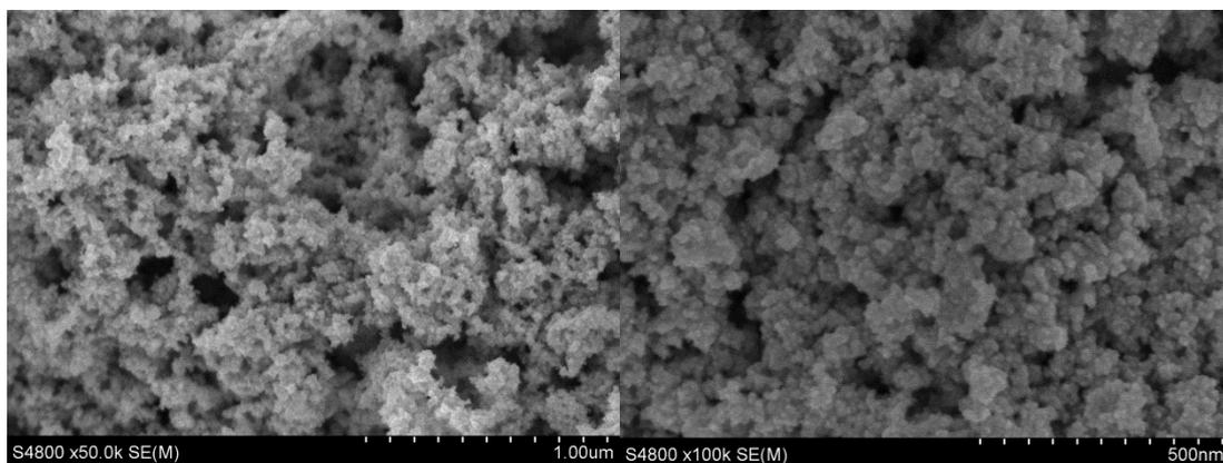
**Fig. S6** FE-SEM patterns of pure Pd NPs with different magnification, left (50k), right (100k).
