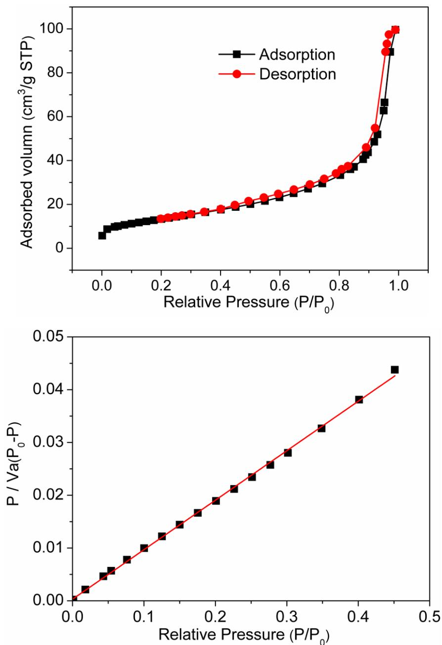
**Fig. S7** Adsorption-desorption isotherms of nitrogen reveal the mesoposity of [PYD]@Pd (up).
