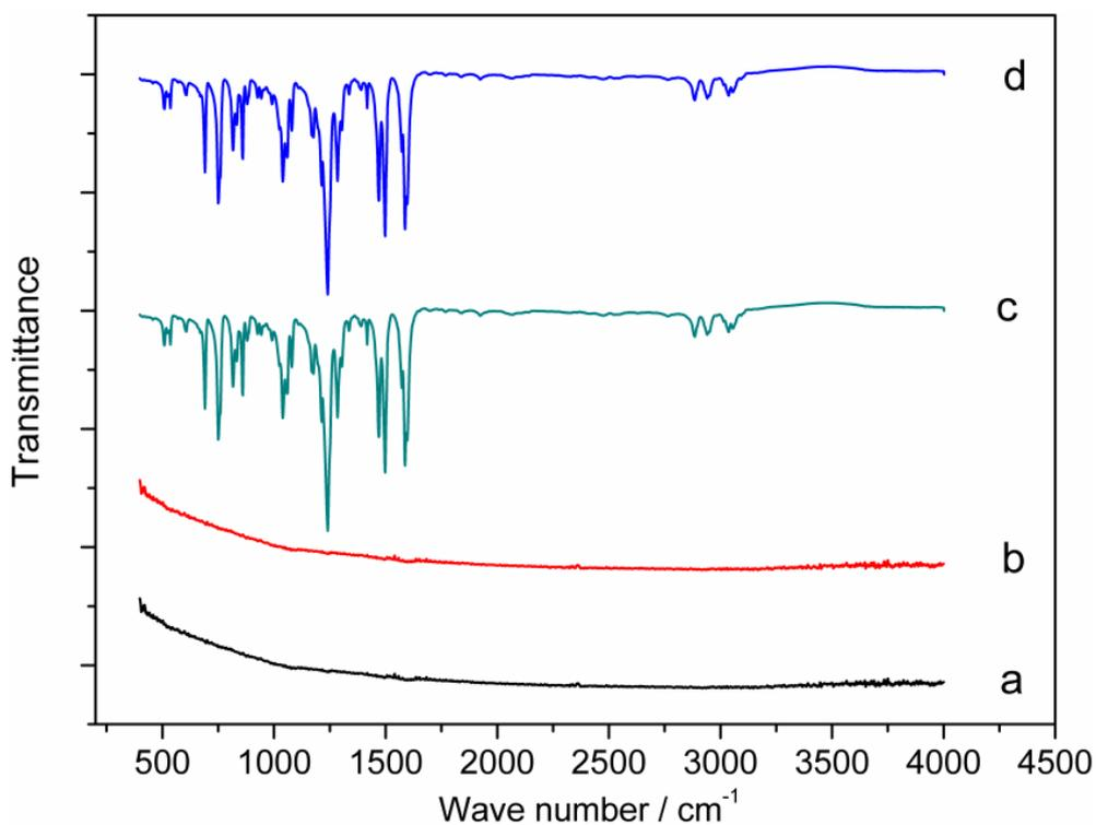
**Fig. S5** FT-IR spectra of [PYD]@Pd (a), pure PYD (c), pure Pd NPs after physical adsorption of PYD (d), (d) after washed with MeCN (b).
