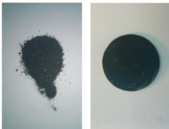
**Fig. S4** Pure Pd NPs before (left) and after (right) press.
