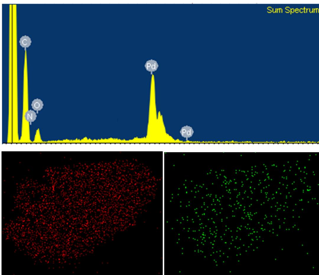
**Fig. S9** The EDX spectrum of [PYD]@Pd after used for 15 times (up); X-ray atomic mapping of the elements of the [PYD]@Pd (down), red and green colours represent Pd and C atoms, respectively.
