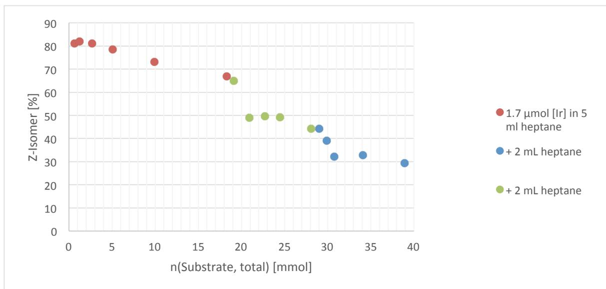
The photoisomerization of (*E*)-3-phenylallyl acetate (**15**) could also be performed at ambient temperatures. The microreactor system was set up as above. Instead of heating to 90 °C, the microreactor was held at a constant temperature of 19 °C through a water cooling system. The flowrate of substrate solution and catalyst solution was set to 50  $\mu\text{L}/\text{min}$ .
