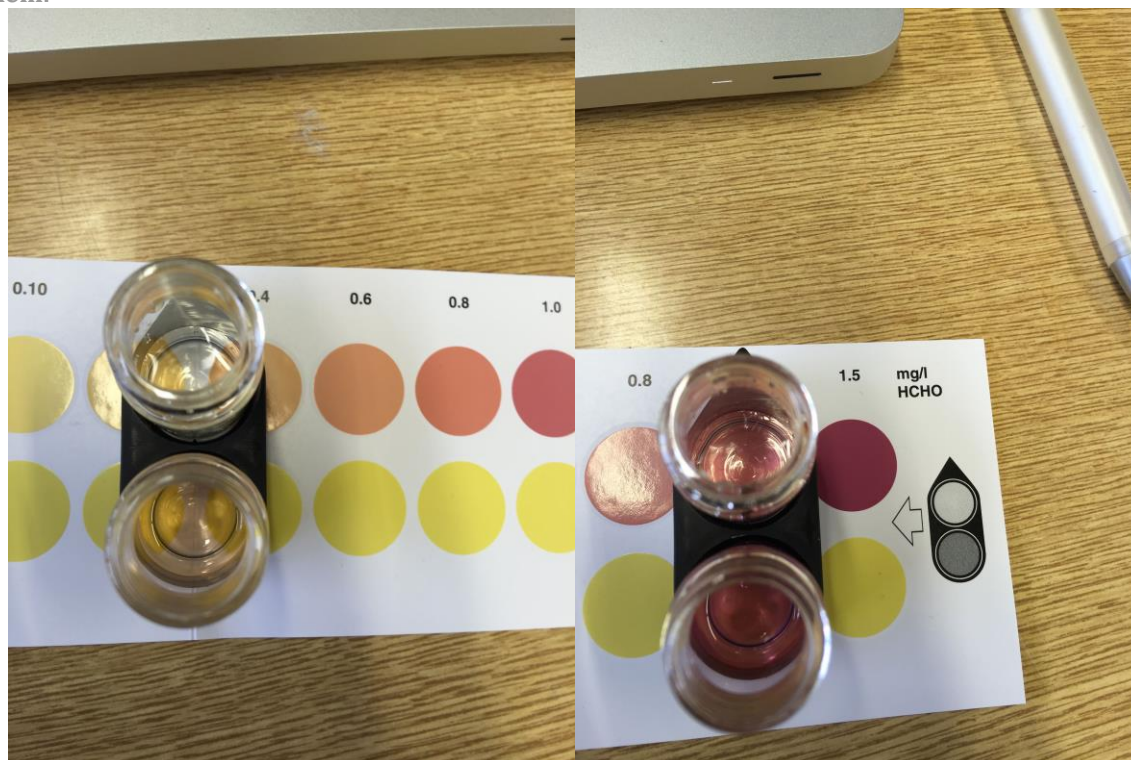
SI-Figure 9: Colorimetric determination of the residual formaldehyde content after 24 h of decontamination experiments with 0.1 mol% [\text{RuCl}_2(\text{p-cymene})]_2 at 95 °C at pH=4-5 (left) and pH=3 (right).
