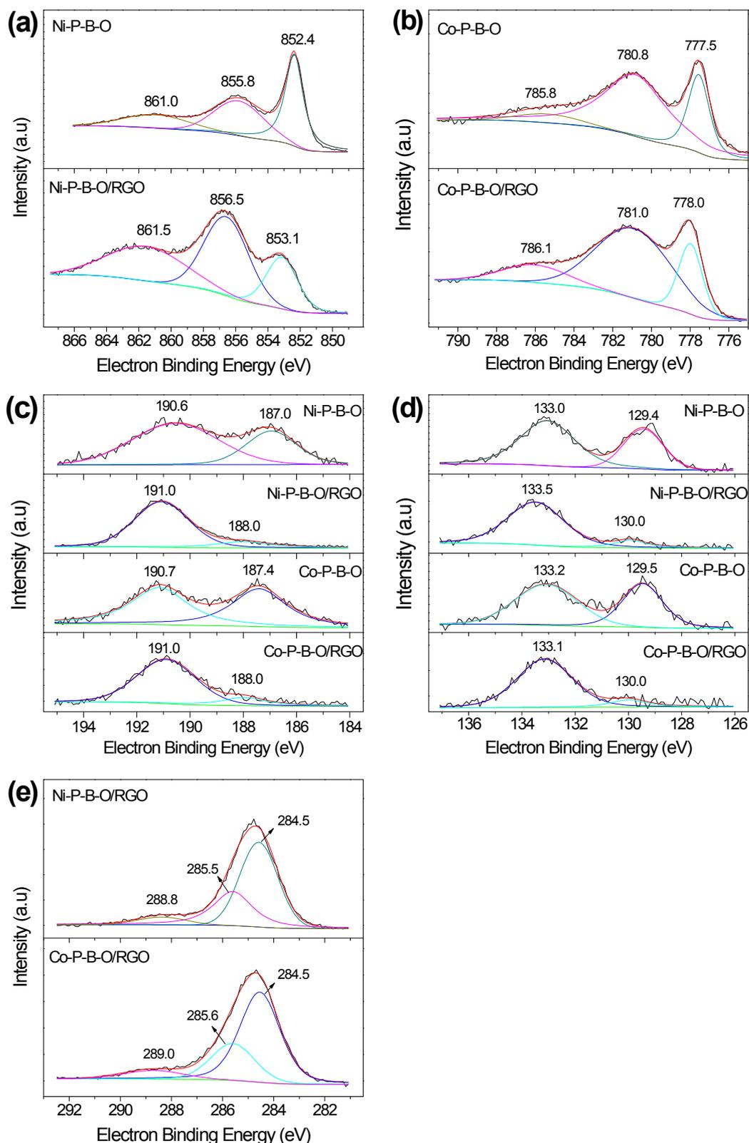
**Fig. S1** XPS spectra of (a) Ni 2p, (b) Co 2p, (c) B 1s, (d) P 2p and (e) C 1s levels of Ni-B-P-O, Ni-B-P-O/RGO, Co-B-P-O and Co-B-P-O/RGO catalysts
