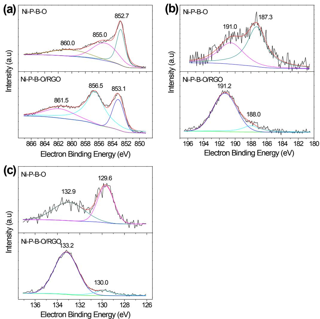
**Fig. S2** XPS spectra of (a) Ni 2p, (b) B 1s and (c) P 2p levels of the used Ni-B-P-O and Ni-P-B-O/RGO catalysts
