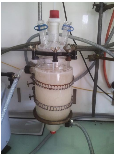
Figure 2: 3-L glass reactor for the preparation of 1,4-D-sorbitan 2 on the large scale.
