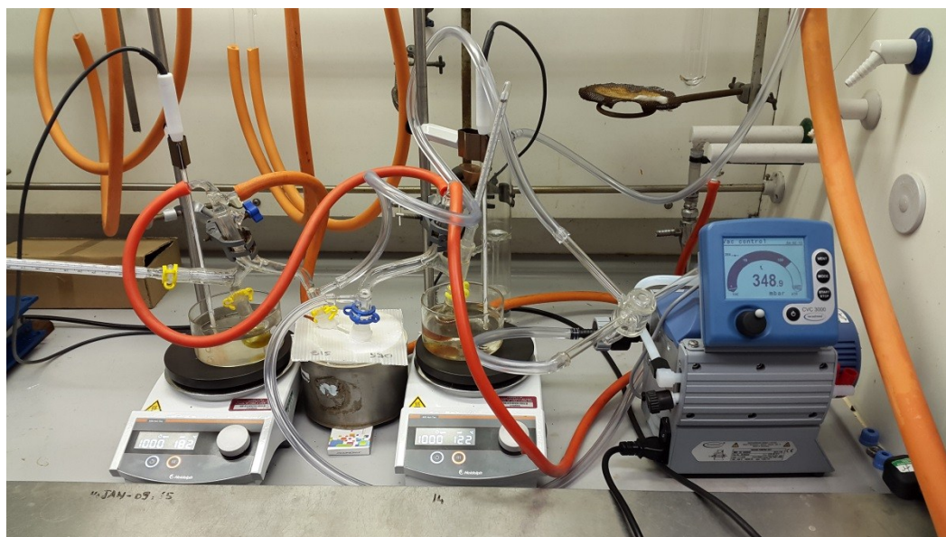
Figure S16. Experimental apparatus for the HTID of 1,3-PDO in the presence of 1 and a base, in ionic liquids, towards selective production of propionaldehyde.
