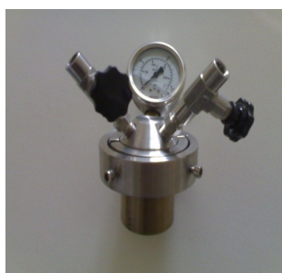
Figure S6. The home-designed reactor for 5-HMF production.
