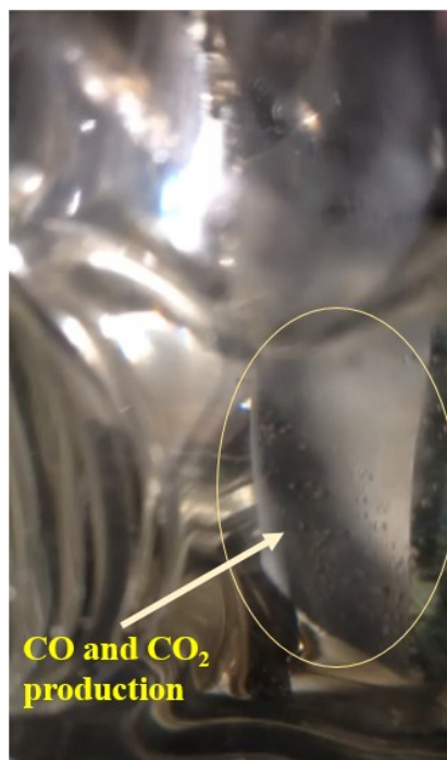
SI-Fig.10 Photoimage of photoanode cell for the C@Cr-SrTiO 3 /TiO 2 NTPC under the visible light irradiation in a 0.5 mol L -1 KOH aqueous solution with 0.1 mol L -1 glucose solution.
