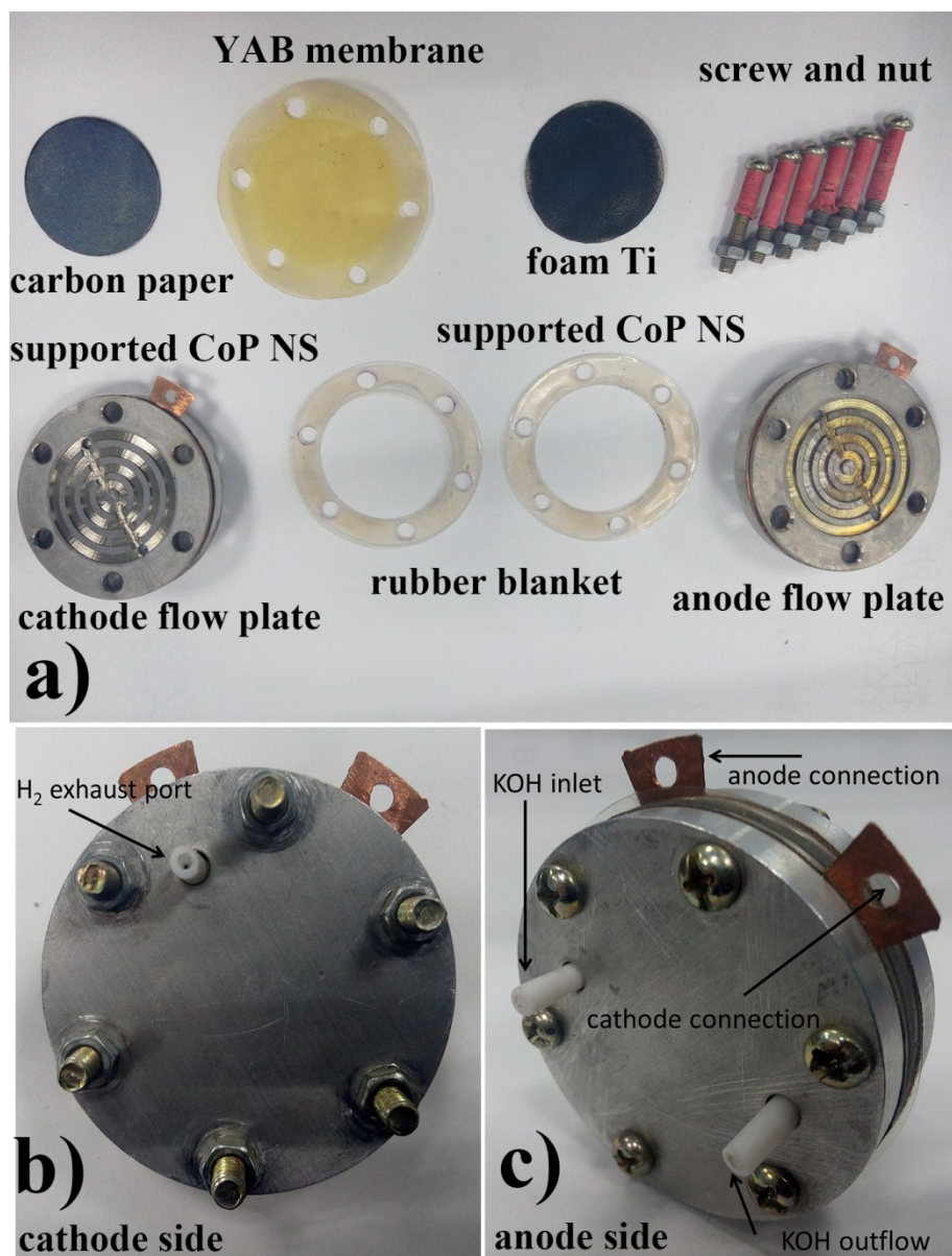
Fig. S9 Potograph of a) AEMWE cell configuration, b) cathode side and c) anode side of the electrolytic cell.
