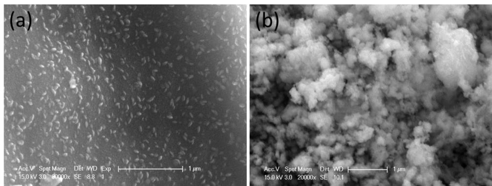
Fig. S6 SEM images of the as-synthesized HT product (a) and  $\text{Fe}_{1-x}\text{S}$  particles (b).
