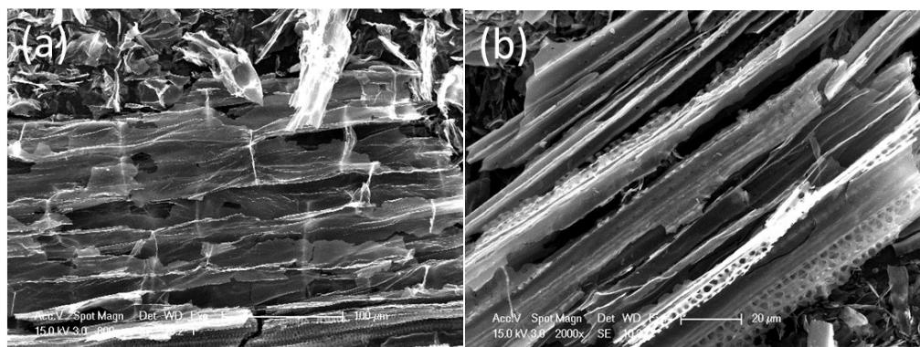
Fig. S7 SEM images of microporous carbon after surface functionalization through acid treatment.
