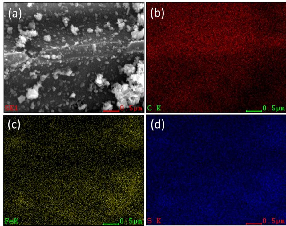
Fig. S3 EDX mapping of  $\text{Fe}_{1-x}\text{S}-\text{MC}$ , suggesting the uniform distribution of the  $\text{Fe}_{1-x}\text{S}$  nanoparticles on MC.
