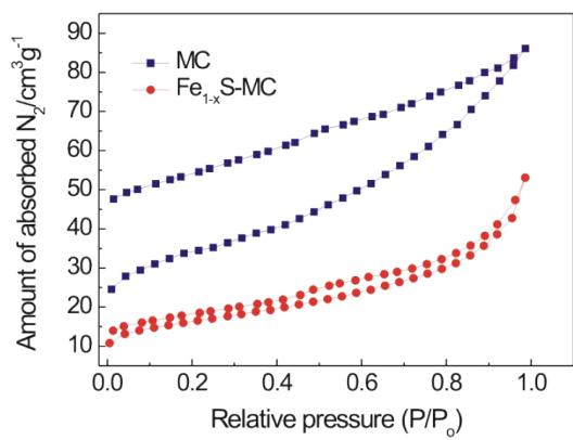
Fig. S2 Nitrogen adsorption–desorption isotherms of microporous carbon and  $\text{Fe}_{1-x}\text{S}-\text{MC}$  at 77 K.
