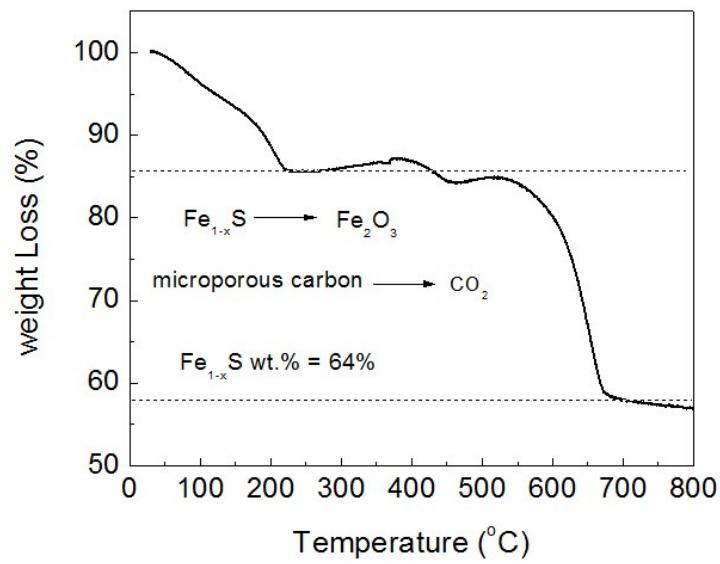
Fig. S4 The TGA curve of the  $\text{FeS}_{1-x}$ -MC nanocomposites.
