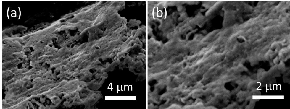
Fig. S8 SEM images of the  $\text{Fe}_{1-x}\text{S}$ -MC nanocomposite after 200 LIB charging/discharging cycles at 100  $\text{mA g}^{-1}$ .
