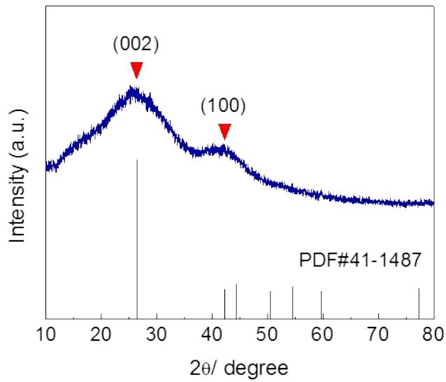
Fig. S5 XRD pattern of microporous carbon.
