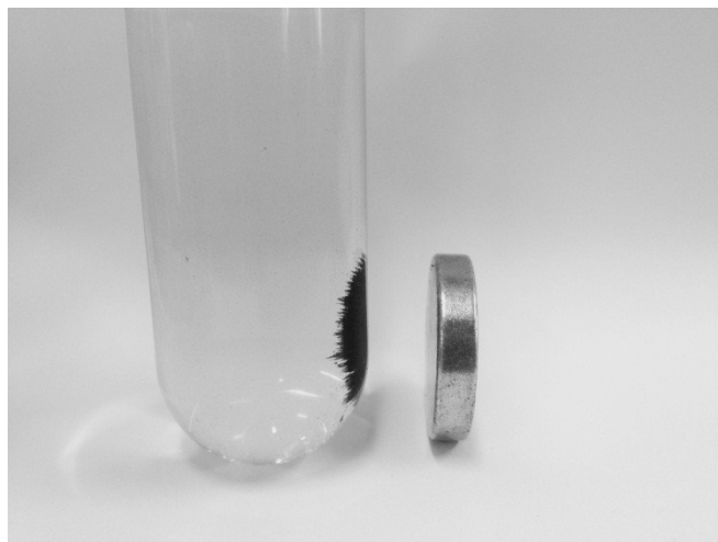
Figure S8. Magnetic separation of the catalyst after reaction.
