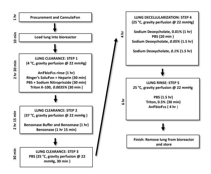
**Supplemental Figure 2** : Flow diagram of proposed decellularization procedure. Total time for the procedure is 16 hours and 35 minutes. Please refer to Table 1 for additional details.
