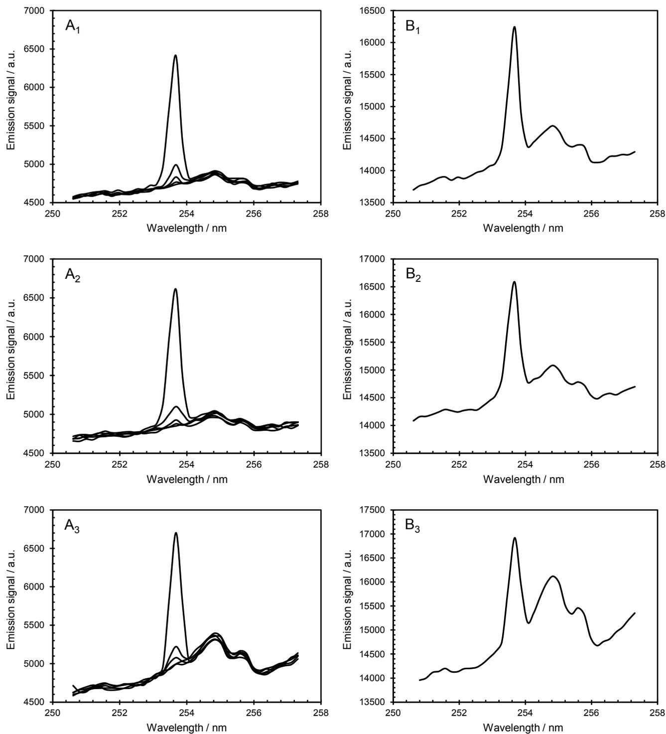
ESI 3. Episodic (A<sub>1</sub>-A<sub>3</sub>) and total emission spectra (B<sub>1</sub>-B<sub>3</sub>) of Hg recorded in 3 successive days under the optimum operating conditions in SICV- $\mu$ CCP-OES for a solution of 0.04 ng mL<sup>-1</sup> Hg (1 ng Hg in 25 mL). Optimal operating conditions: 8 min sonication time; 0.2 mol L<sup>-1</sup> formic acid; 10 W plasma power; 100 mL min<sup>-1</sup> Ar flow rate; 0.8 mm observation height.
